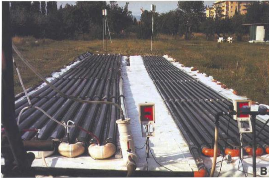
Figure 12 - The plexiglass tubular photobioreactor. The tube loops are placed on a white sheet to help reflect light back into the reactor (Tredici & Materassi 1992).
