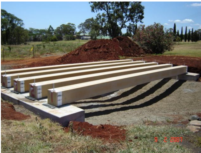
Figure 1 Hybrid Composite Bridge Beams
