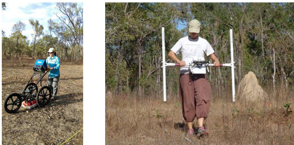
Figure 3. 3 Kelsey Lowe with the ground penetrating radar and gradiometer behind the officers' quarters (Photograph Bateman 2016)
