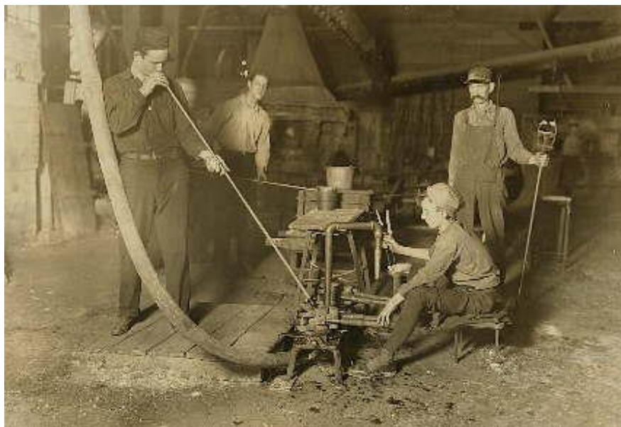
Figure 5. 5 Mouth-blown shop crew from West Virginia working at the mould in 1908 (Lindsey 2015a)
