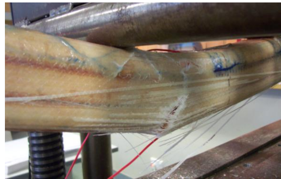
FIGURE 07: Failure of specimen 3LSW-WF
