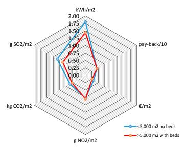
**Figure 2.** Potential of energy saving derived from improvement of air conditioning and heating systems (HVAC) systems.
