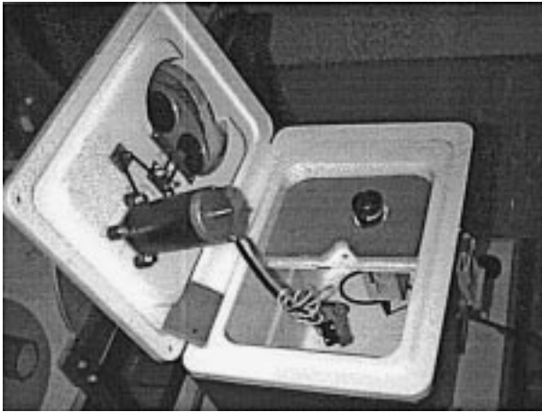
FIG. 2. Stepper motor used to turn a filter wheel assembly, which is located above the camera lens when the lid is closed. This Peltier-cooled housing is also shown in the background of Fig. 1.
