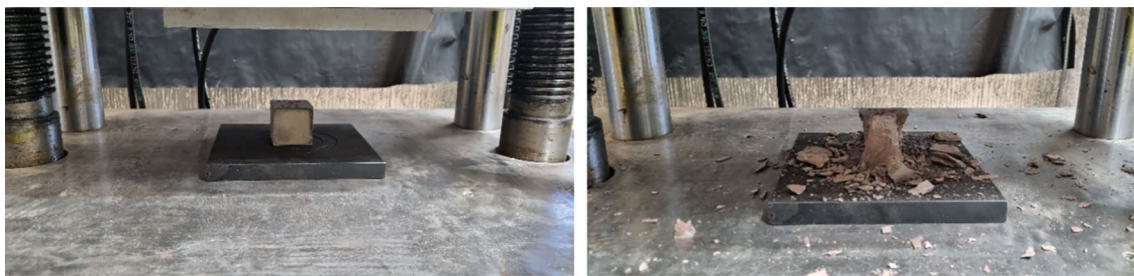
Fig. 2 A sample before and after the UCS test
