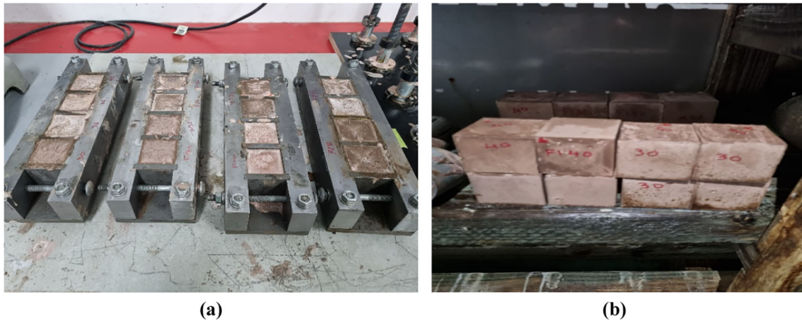
Fig. 1 a Grout preparation and b a view of UCS samples in the curing room
