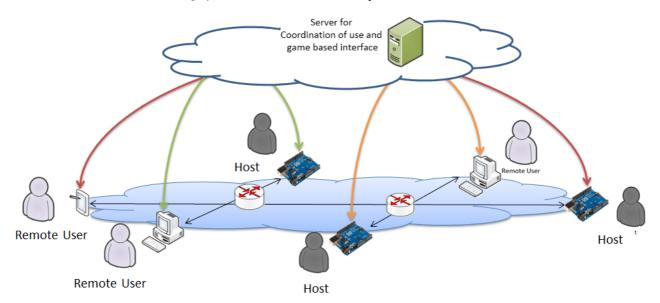
Figure 3. The distributed RAL architecture
