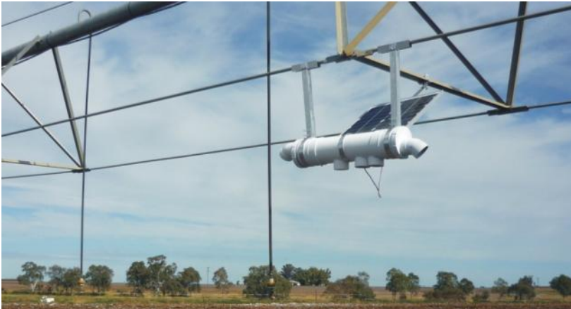
Figure 2. PA in Horticulture - Spatial and real time crop performance data for adaptive control and variable rate technology. Sensors include crop canopy temperature, Vis & IR (NDVI), crop height 3/4G telemetry coupled with a mini computer to log data and transmit to; PC, the cloud or irrigation controller.
