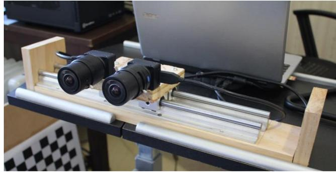
*Figure 7.22: Stereo camera system used for capturing custom stereo images. The setup contains two FLIR Chameleon CM3-U3-13S2C-CS cameras fitted with Computar A4Z2812CS-MPIR FISHEYE lenses (with manually variable focal length 2.8mm-10mm and iris) mounted on a hand built stereo camera rig.*
