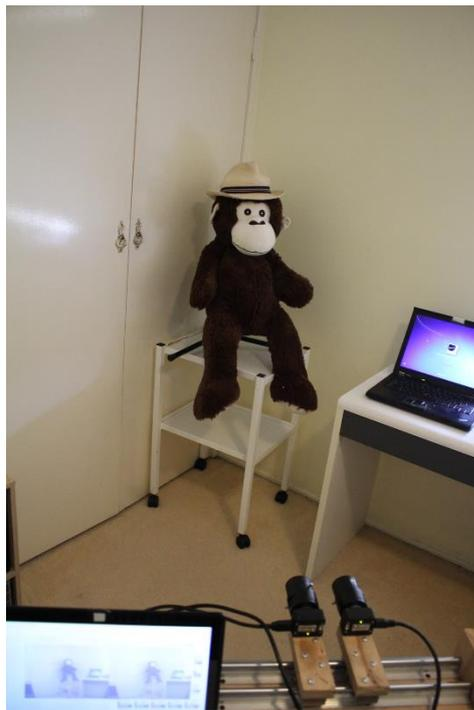
*Figure 7.23: A static image being captured by using the custom-built stereo camera system.*
