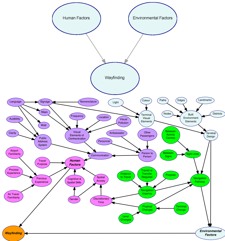
Figure 1: The Wayfinding Bayesian Network model (WBNM), comprising three interconnected subnetworks (top) which expand to a full model (bottom) (Farr et al. , 2014).
