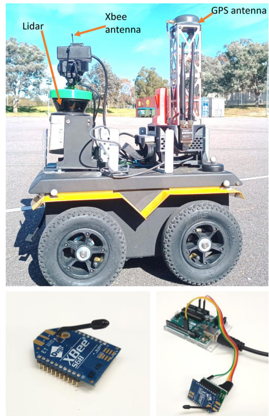
FIGURE 8 | The Jackal mobile robot used for the radio source localization and field tests is shown on top. The XBee modems are mounted on the robot with the help of a plastic bracket. The XBees are placed as high as possible on the robot to minimize ground reflections. The XBee modem and the Arduino attachment used for the testing are shown at the bottom.
