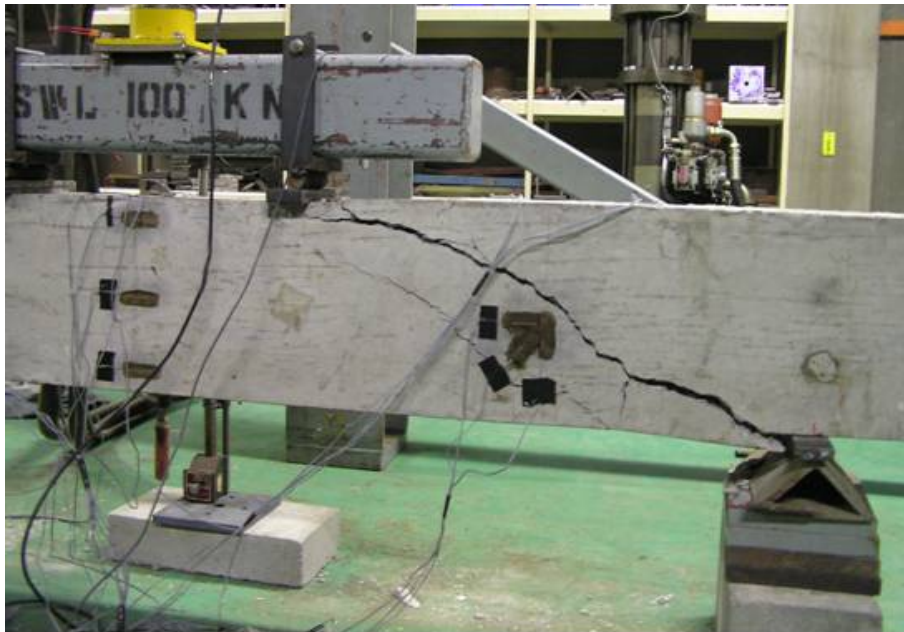
Figure 4.6. Failure of control specimen EPT11 (Right hand side of the specimen is shown)
