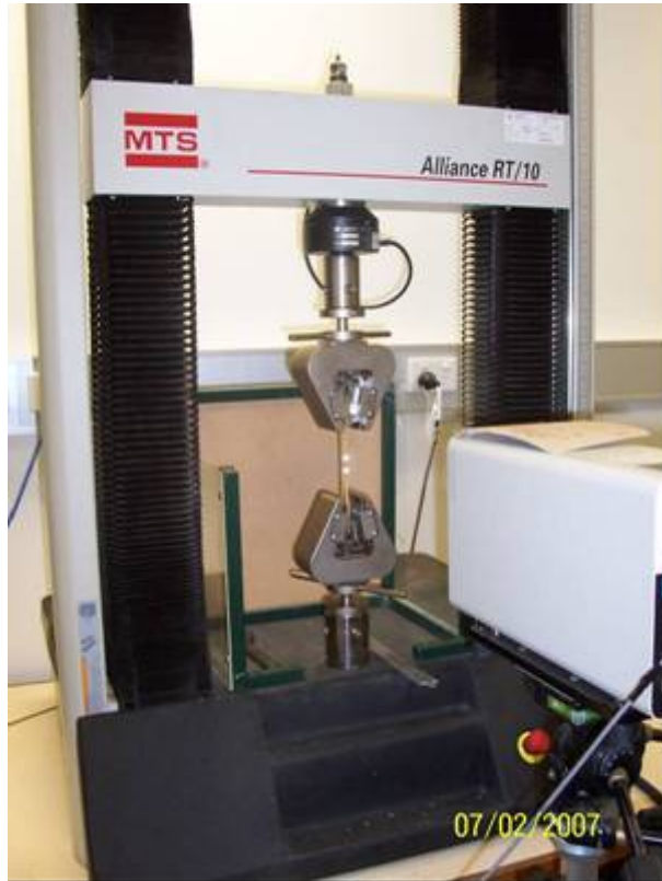
(a) Specimen fixed in the MTS machine
