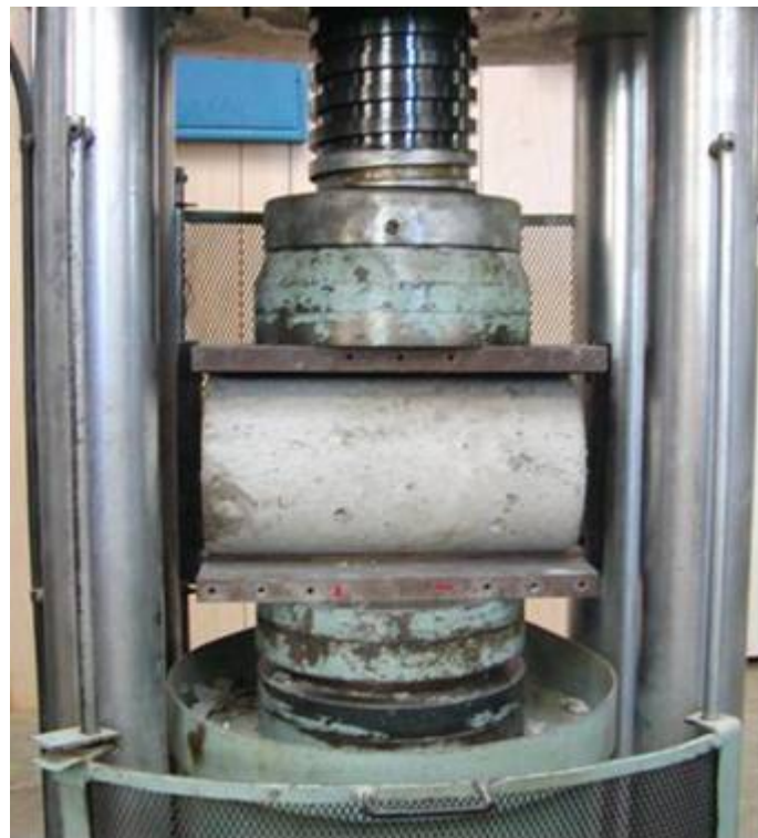
Figure 3.6. Testing of indirect tensile strength of the concrete
