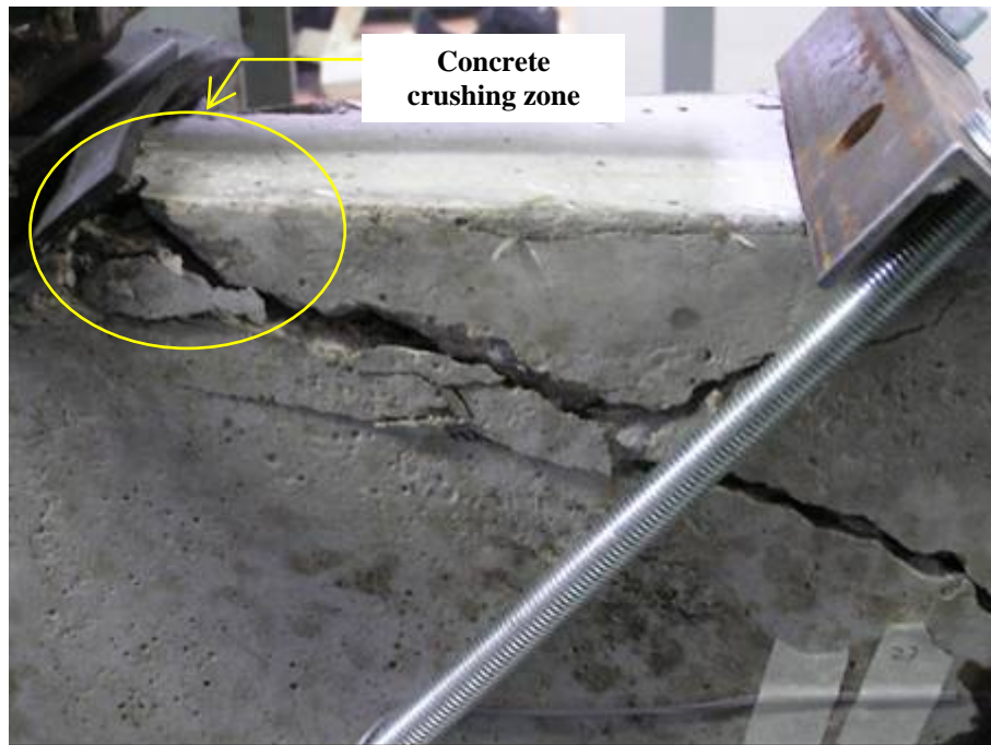
Figure 4.28. Localised concrete failure near loading point of ECL36 and ECL37
