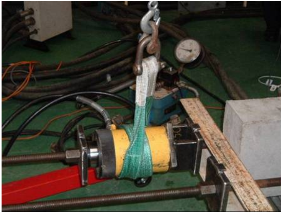
Figure 3.20. Hydraulic jacking system used for post-tensioning at the ‘active’ end of the specimen
