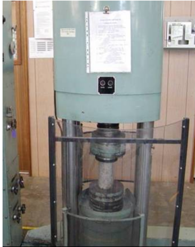
Figure 3.5. Testing of compressive strength of the concrete
