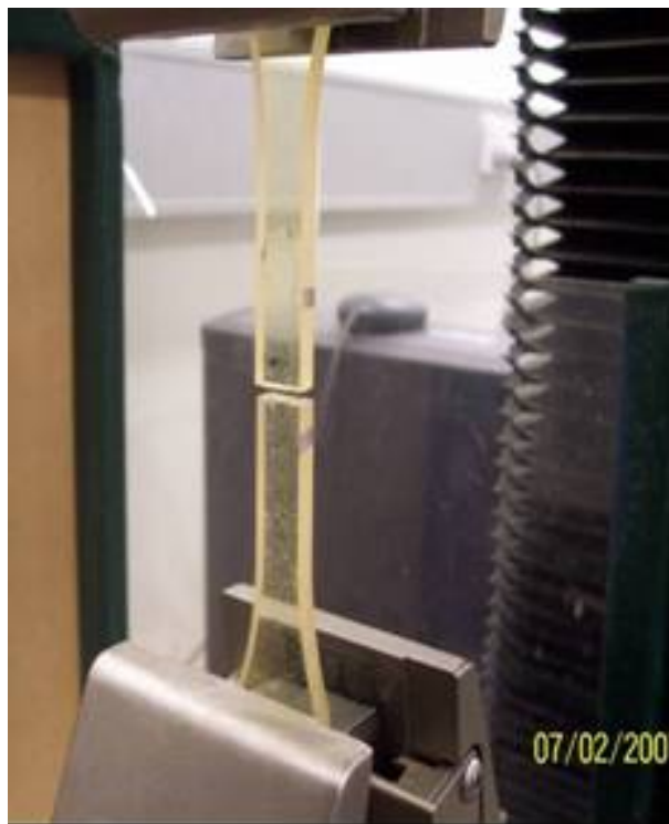
(b) Failure of the specimen
