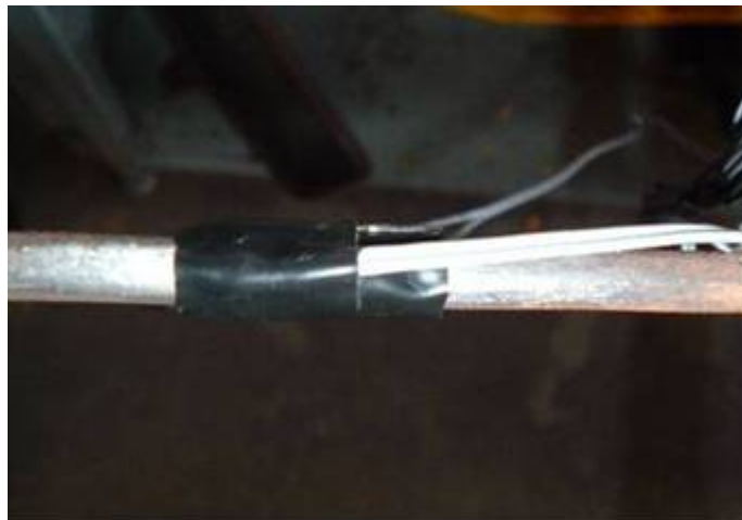
Figure 3.12. Strain gauge attached in shear reinforcement
