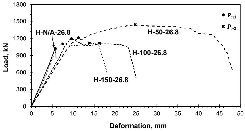
Fig. 5. Load–deformation behavior of group A columns
