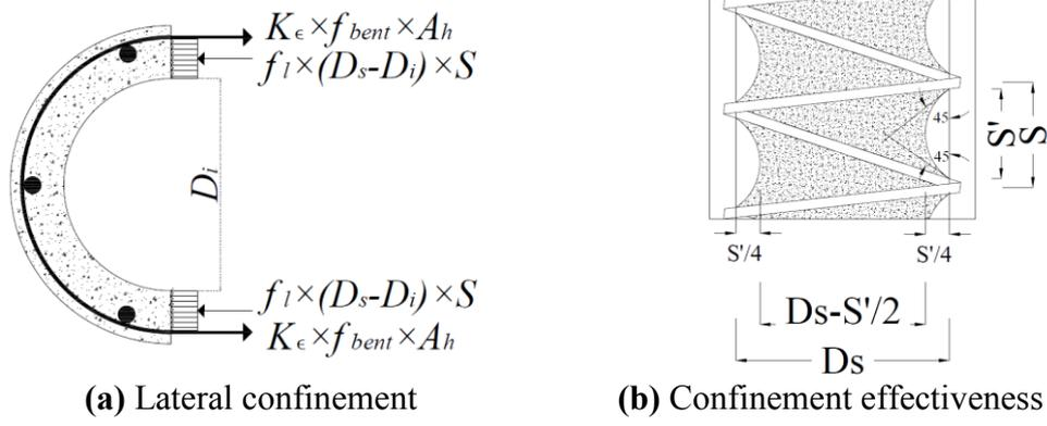
**Fig. 12.** Lateral-confinement mechanism and confinement effectiveness factor
