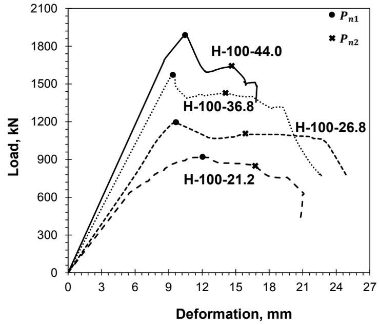
**Fig. 9.** Load–deformation behavior of group B columns
