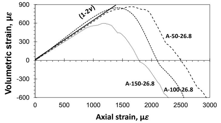
(b) Volumetric-strain versus axial-strain behavior
