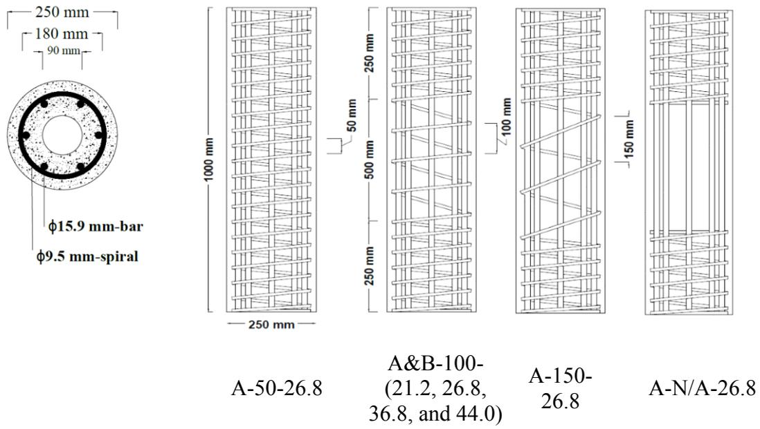
**Fig. 2.** Typical cross section of columns and lateral spiral details
