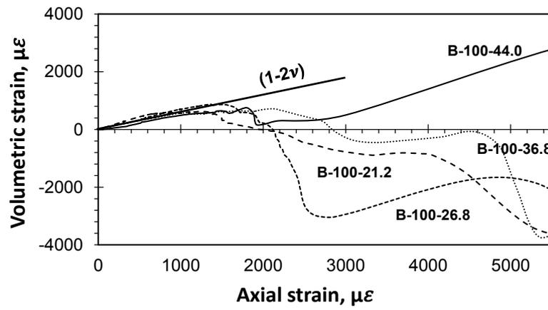
**Fig. 11.** Volumetric strain versus axial strain for Group B columns
