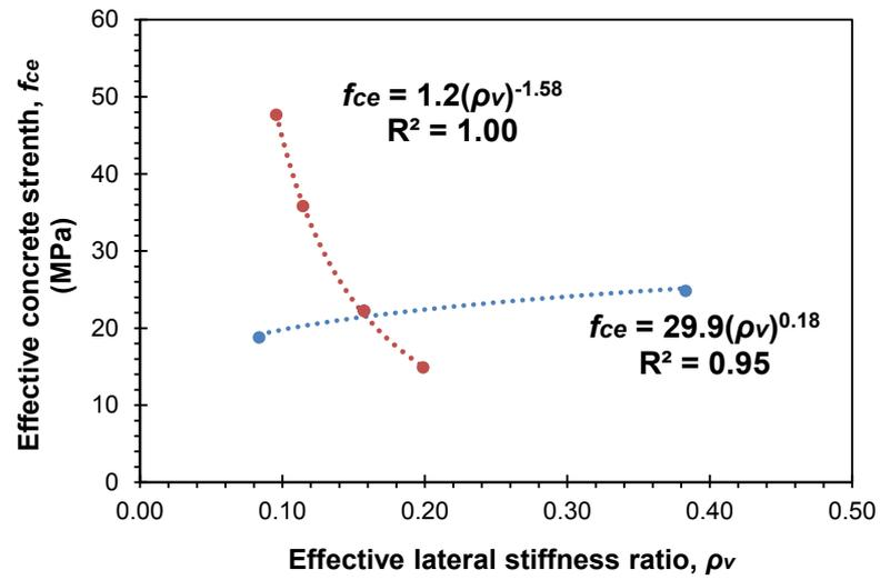
**Fig. 13.** Influence of lateral stiffness ratio ( $\rho_v$ ) on the effective concrete strength ( $f_{ce}$ )
