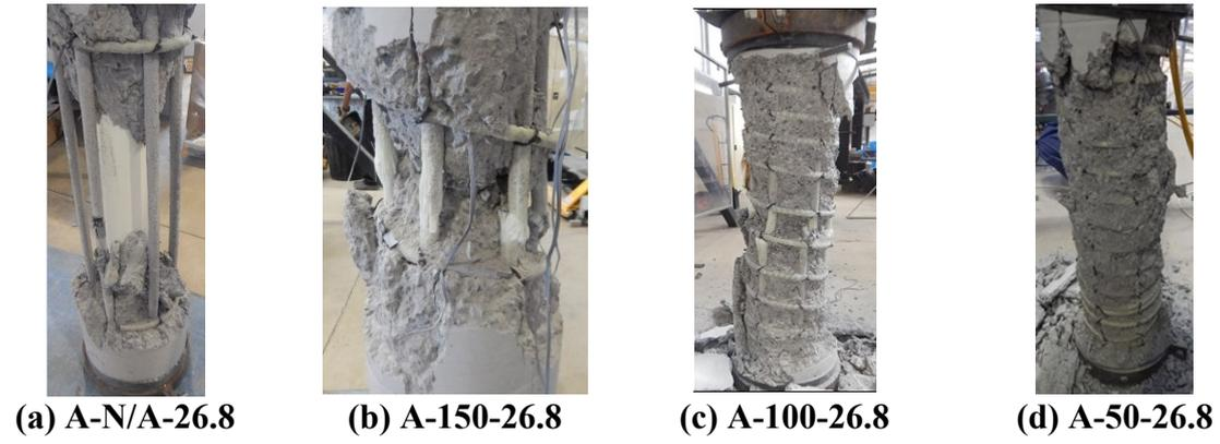
**Fig. 4.** The final failure of the columns in Group A
