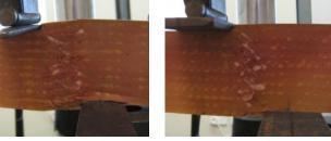
(c) 20 mm plate (d) 30 mm plate Figure 7. Failure of AS-SW-E with different plate width.
