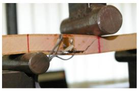
Figure 4. Failure behaviour of specimen AS-SW-F.
