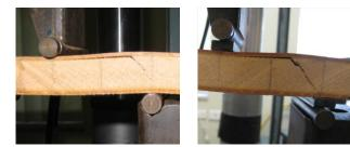
(a) no plate (b) 10 mm plate Figure 6. Failure of AS-SW-F with different plate width.
