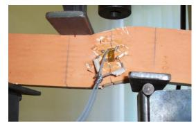
Figure 5. Failure behaviour of specimen AS-SW-E.
