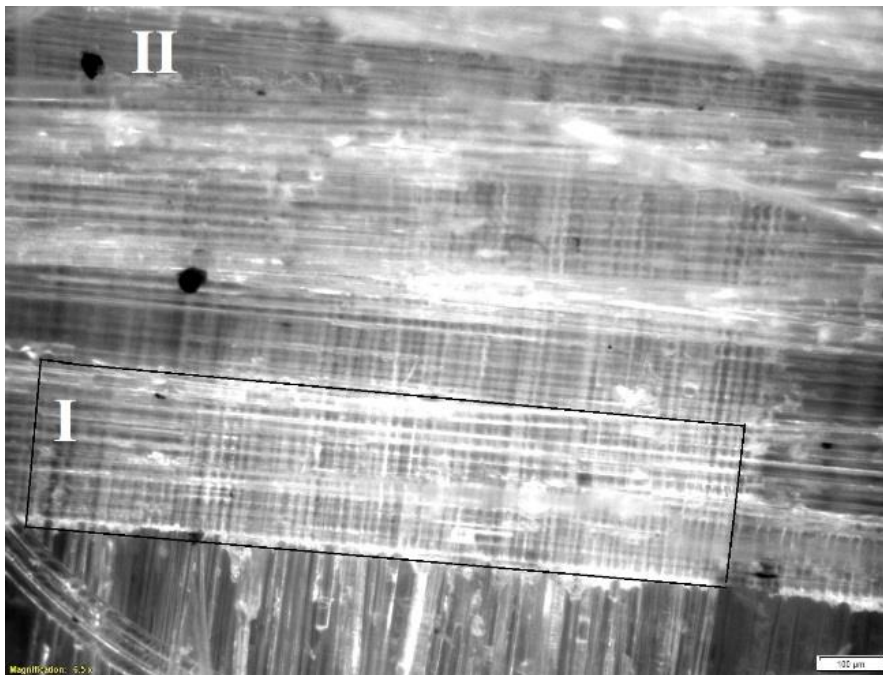
Figure 5-2 Microscopic view of a DCB test specimen; brighter microcrack spots (Region I) and propagation of delamination crack (Region II)
