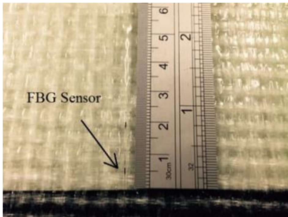
Figure 4-3 Location of Embedding FBG sensor in the specimen
