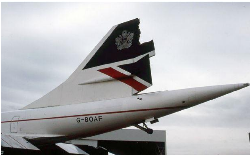
Figure 2-18 Losing upper rudder of upper rudder of Concorde G-BOFA due to delamination damage. The photograph was taken at Sydney by Ken Watson, at that time a Qantas Engineer ( http://www.concordesst.com/latestnews_02_1.html )
