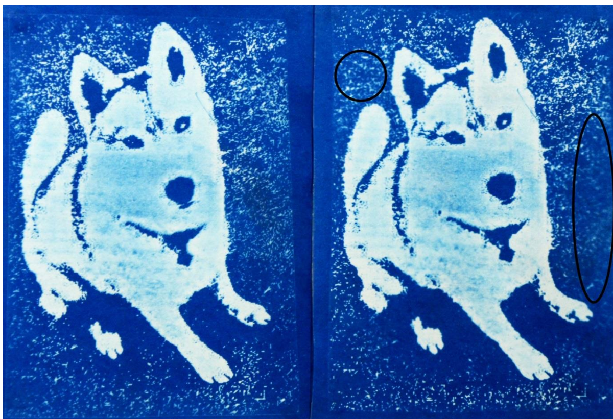
Figure 10 - Photograms using transparent prints. The image on the left was produced in direct sunlight in less than five minutes. Most of the image is relatively clear. The image on the right was produced under shade with diffuse radiation and took five to ten minutes to produce. Parts of the image are blurred (see highlighted areas); however this is not due to image movement.
