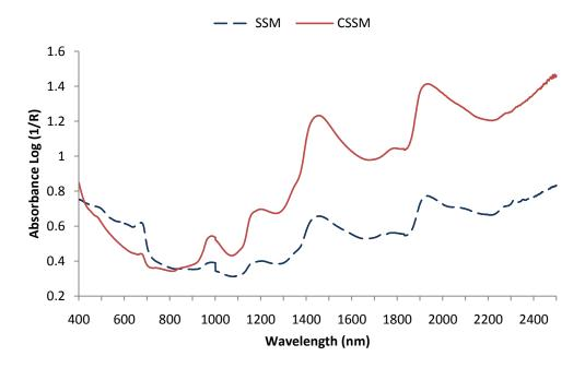
Figure 7.10: Comparison of typical absorbance spectrum between SSM and CSSM
