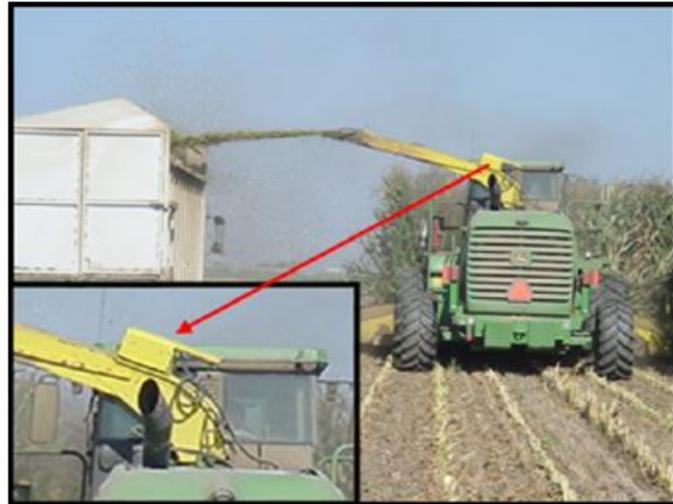
**Figure 8.4: Location of a mounted spectrometer to measure crop moisture in forage (Digman & Shinnars 2008)**
