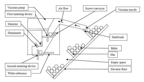
Figure 8.10: Schematic diagram of the QMSS with ASM
