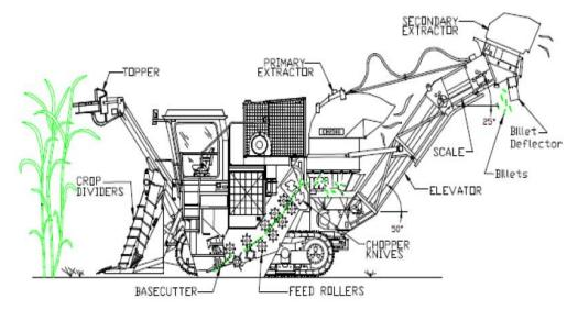
Figure 2.4: Typical sugarcane harvester (Caryn et al. 2002)
