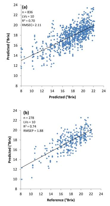
Figure 7.7: Scatter plots of reference versus predicted °Brix for individual spectrum data by the SSM: (a) calibration model; (b) prediction model
