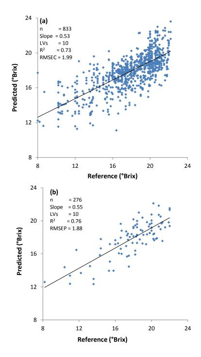
Figure 6.9: Scatter plots of reference versus predicted °Brix for individual spectrum data by the CSSM: (a) calibration model; (b) prediction model
