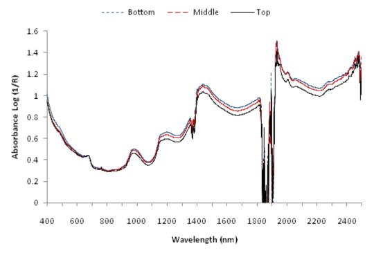
Figure 6.1: Typical absorbance spectra for bottom, middle and top sections as measured by the FRS
