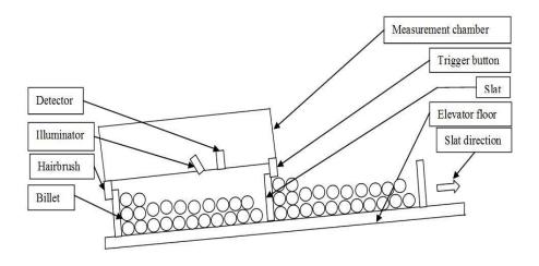
Figure 8.8: Schematic diagram of the QMSS with DSM
