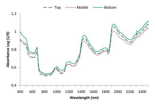
Figure 7.2: Typical absorbance spectra of SSM for different stalk sections as measured by the FRS
