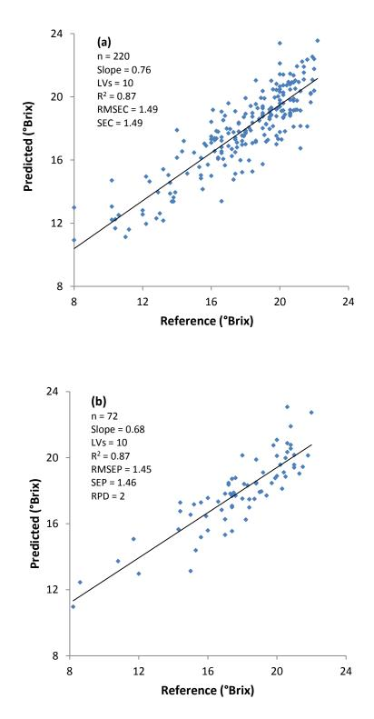
Figure 6.7: Scatter plots of reference versus predicted °Brix for absorbance spectral data by the CSSM: (a) calibration model; (b) prediction model
