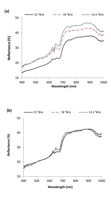
Figure 7.3: Typical reflectance spectra for sugarcane internodes at different °Brix values: (a) raw reflectance spectra; (b) reflectance spectra pre-processed with MSC
