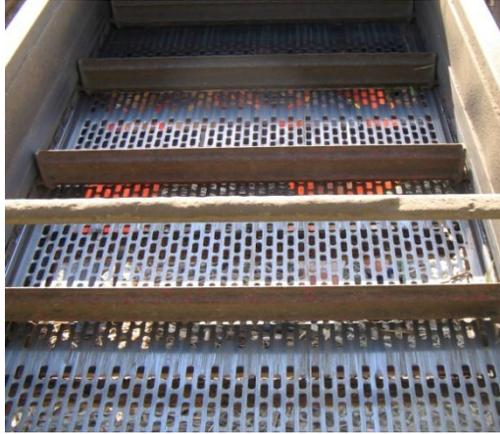
**Figure 8.5: Typical slat arrangement on the elevator of a sugarcane harvester**
