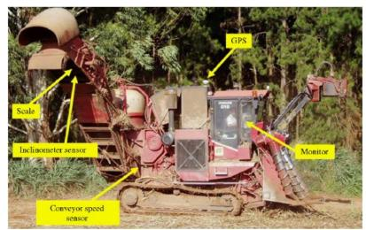
Figure 2.11: A sugarcane harvester equipped with components of yield monitoring system (Magalhães & Cerri 2007)
