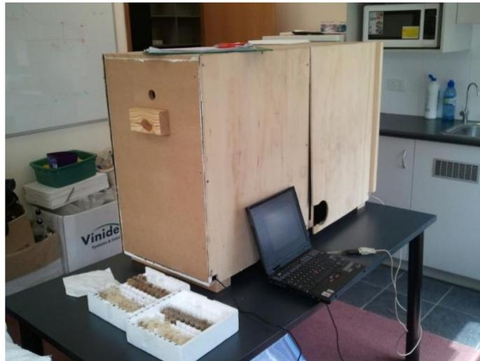
**Figure 4.4: Light-proof measurement box in use**
