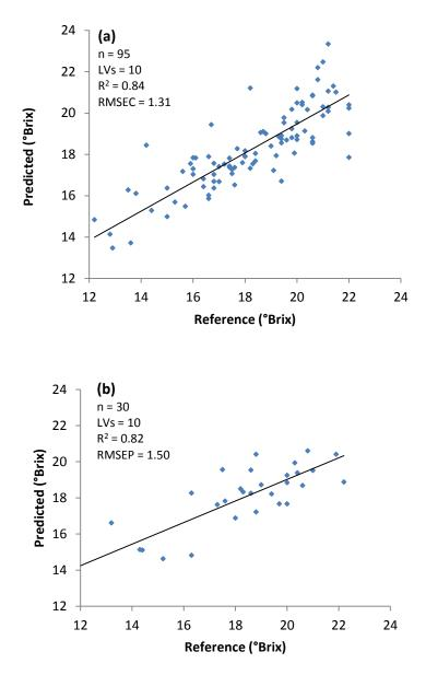
Figure 7.9: Scatter plots of reference versus predicted °Brix by SSM in the wavelength range of 400 to 1800 nm: (a) calibration model; (b) prediction model
