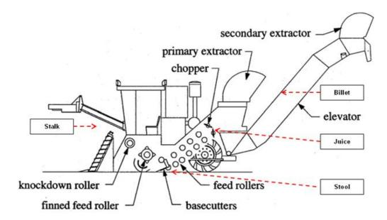
Figure 8.1: Location from which possible samples could be obtained
