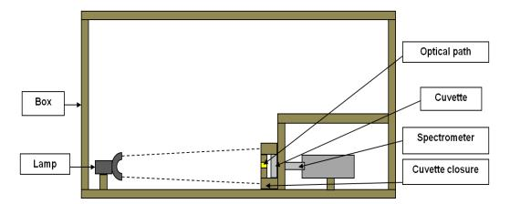
Figure 4.6: Simplified diagram of the transmittance measurement inside the measurement box
