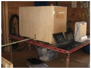
Figure 4.9: The whole stalk sample being scanned using spectroscopic method inside the measurement box
