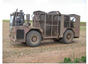
Figure 2.5: Haul-out truck to carry harvested sugarcane from a harvester to rail sidings
