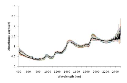
Figure 6.16: Typical absorbance spectra collected by the FRS after being treated with MSC method
