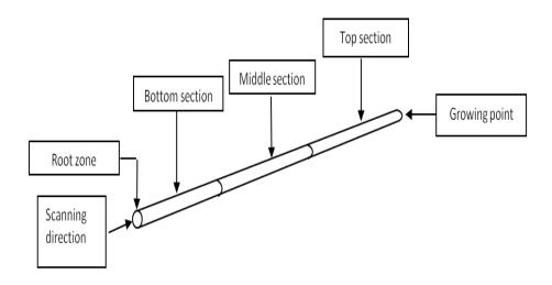
Figure 4.8: The division of fresh sugarcane stalks into three main sections
