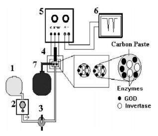
Figure 2.14: Flow injection manifold of biosensor for the determination of sucrose: (1) buffer reservoir, (2) peristaltic pump, (3) injector, (4) electrochemical cell, (5) potentiostat, (6) record, (7) waste reservoir (Kennedy et al. 2007)
