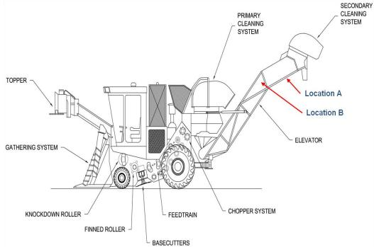
Figure 8.6: Proposed locations of two measurement chambers
