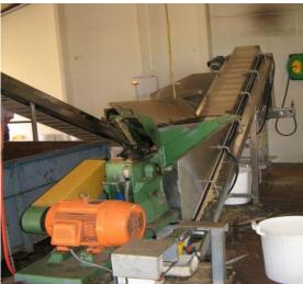
Figure 4.13: Sugarcane disintegrator used to fibrate stalk samples
