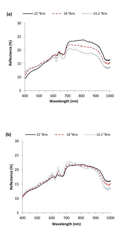
Figure 6.6: Typical reflectance spectra of CSSM at different °Brix values: (a) raw reflectance spectra; (b) reflectance spectra pre-processed with MSC
