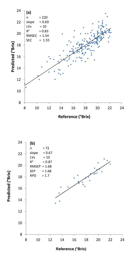
Figure 7.6: Scatter plots of reference versus predicted °Brix for absorbance spectral data by the SSM: (a) calibration model; (b) prediction model
