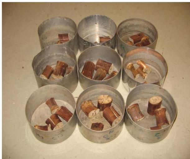
**Figure 4.12:** Cut section of internode samples which have been oven dried
