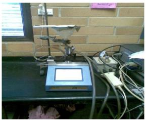
Figure 2.6: A typical desktop refractometer for measuring sugarcane °Brix
