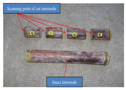
Figure 4.11: Intact internode versus cut internode with scanning positions
