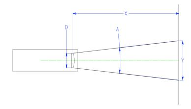
Figure 4.7: Assisted diagram for calculating field-of-view (ASD 2005)
