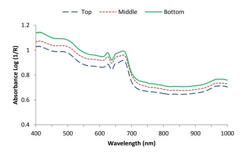
Figure 7.1: Typical absorbance spectra of SSM for different stalk sections as measured by the VNIRS
