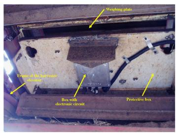
Figure 2.12: Position of a scale set-up on the elevator of the sugarcane harvester from bottom view (Magalhães & Cerri 2007)
