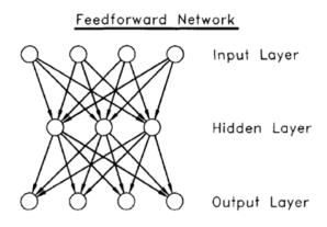
Figure 4.16: Three layers of feed-forward ANN
