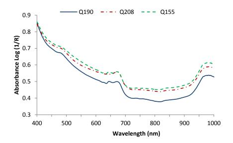
Figure 6.11: Typical absorbance spectra of CSSM for different varieties
