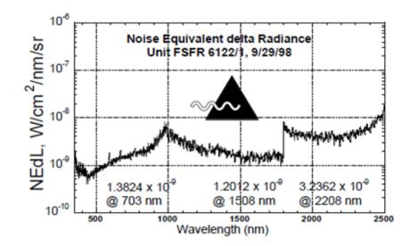
Figure 4.2: Sensitivity figure of FRS as indicated by NeDL (ASD 1999)
