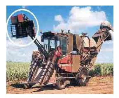
Figure 2.15: Location of the electronic refractometer installed to measure sugarcane juice samples
