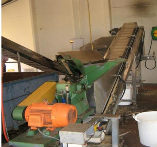
**Figure 4.13: Sugarcane disintegrator used to fibrated stalk samples**
