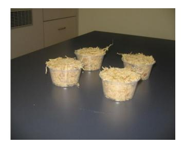
Figure 4.14: Fibrated sugarcane samples for reflectance measurement
