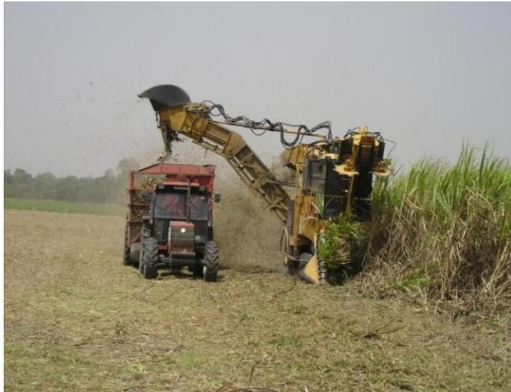
**Figure 2.3: Sugarcane being harvested by a conventional sugarcane harvester**
