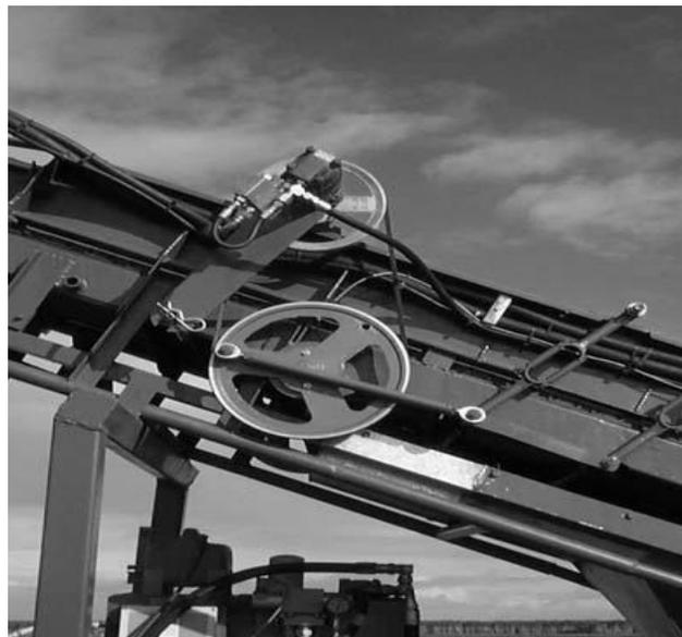
**Figure 8.3: Sampling door and Pitman arm system (Robotham 2000)**
