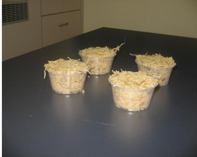
**Figure 4.14: Fibrated sugarcane samples for reflectance measurement**
