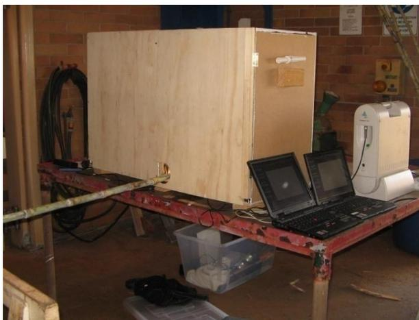
**Figure 4.9: The whole stalk sample being scanned using spectroscopic method inside the measurement box**
