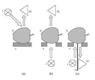
Figure 3.3: Setup for the acquisition of (a) reflectance, (b) transmittance, (c) interactance spectra; (i) the light source, (ii) fruit, (iii) monochromator/detector, (iv) light barrier, (v) support (Nicolai et al. 2007)
