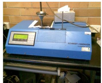
Figure 2.7: A typical desktop polarimeter for measuring sugarcane pol
