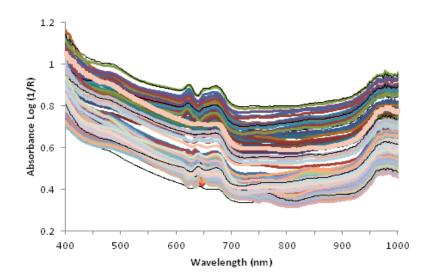
Figure 6.13: Typical raw absorbance spectra for CSSM collected by the VNIRS
