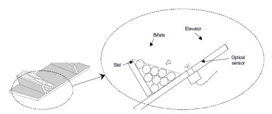
Figure 2.13: Method to detect billets from the elevator floor using optical sensors (Price et al. 2011)
