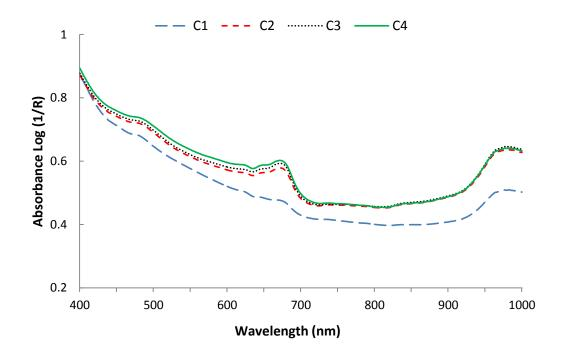
Figure 6.10: Typical absorbance spectral curves of CSSM for each cut section
