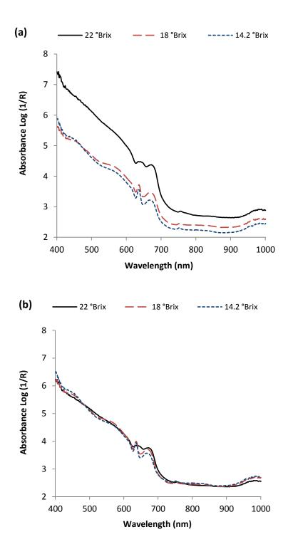
Figure 7.4: Typical absorbance spectra for sugarcane internodes at different °Brix values: (a) raw absorbance spectra; (b) absorbance spectra pre-processed with MSC
