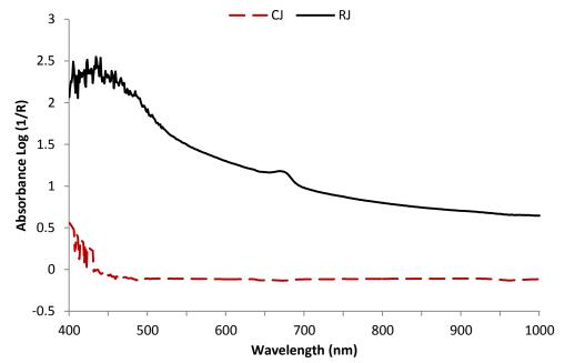
Figure 5.2: Typical absorbance spectra of CJ and RJ as measured by transmittance mode
