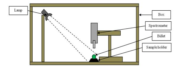
Figure 4.5: Simplified diagram of the reflectance measurement inside the measurement box
