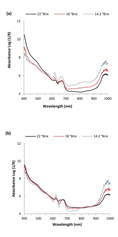
Figure 6.5: Typical absorbance spectra of CSSM at different °Brix values: (a) raw absorbance spectra; (b) absorbance spectra pre-processed with MSC
