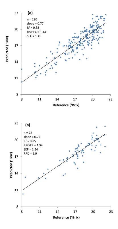
Figure 6.8: Scatter plots of reference versus predicted °Brix for reflectance spectral data by the CSSM: (a) calibration model; (b) prediction model
