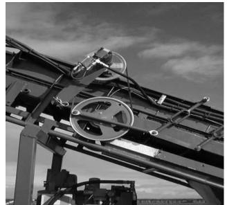
Figure 8.3: Sampling door and Pitman arm system (Robotham 2000)
