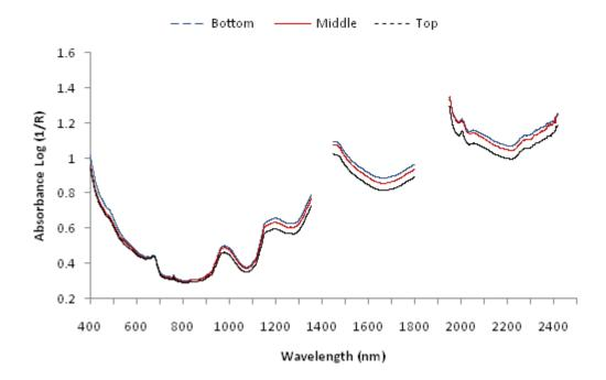
Figure 6.2: Typical absorbance spectra for bottom, middle and top sections as measured by the FRS (without water bands)
