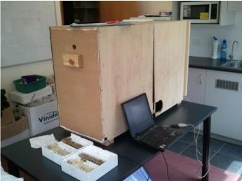
Figure 4.4: Light-proof measurement box in use
