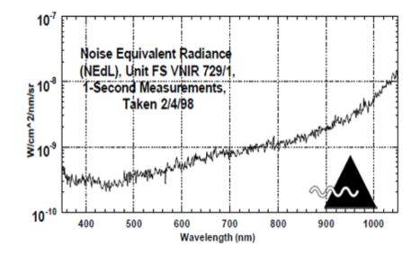
Figure 4.1: Sensitivity figure of VNIRS as indicated by NeDL (ASD 1999)
