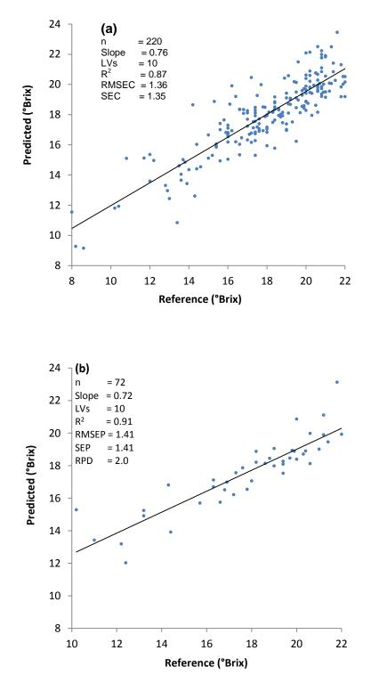
Figure 7.5: Scatter plots of reference versus predicted °Brix for reflectance spectral data by the SSM: (a) calibration model; (b) prediction model
