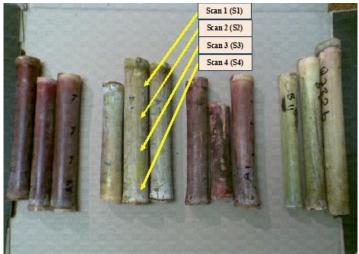
**Figure 4.10: Scanning positions along individual internodes**
