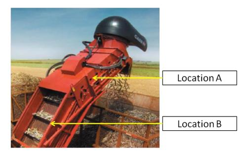
Figure 8.7: Condition of billets on the elevator at the proposed measurement point
