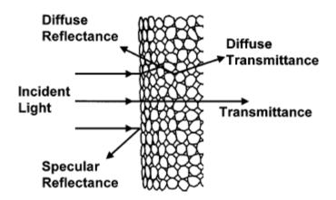
Figure 3.2: Incident light on a fruit results in specular reflectance (gloss), diffuse reflectance, diffuse transmittance, or absorbance (Abbott 1999)
