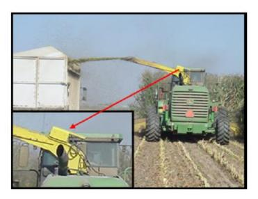
Figure 8.4: Location of a mounted spectrometer to measure crop moisture in forage (Digman & Shinners 2008)
