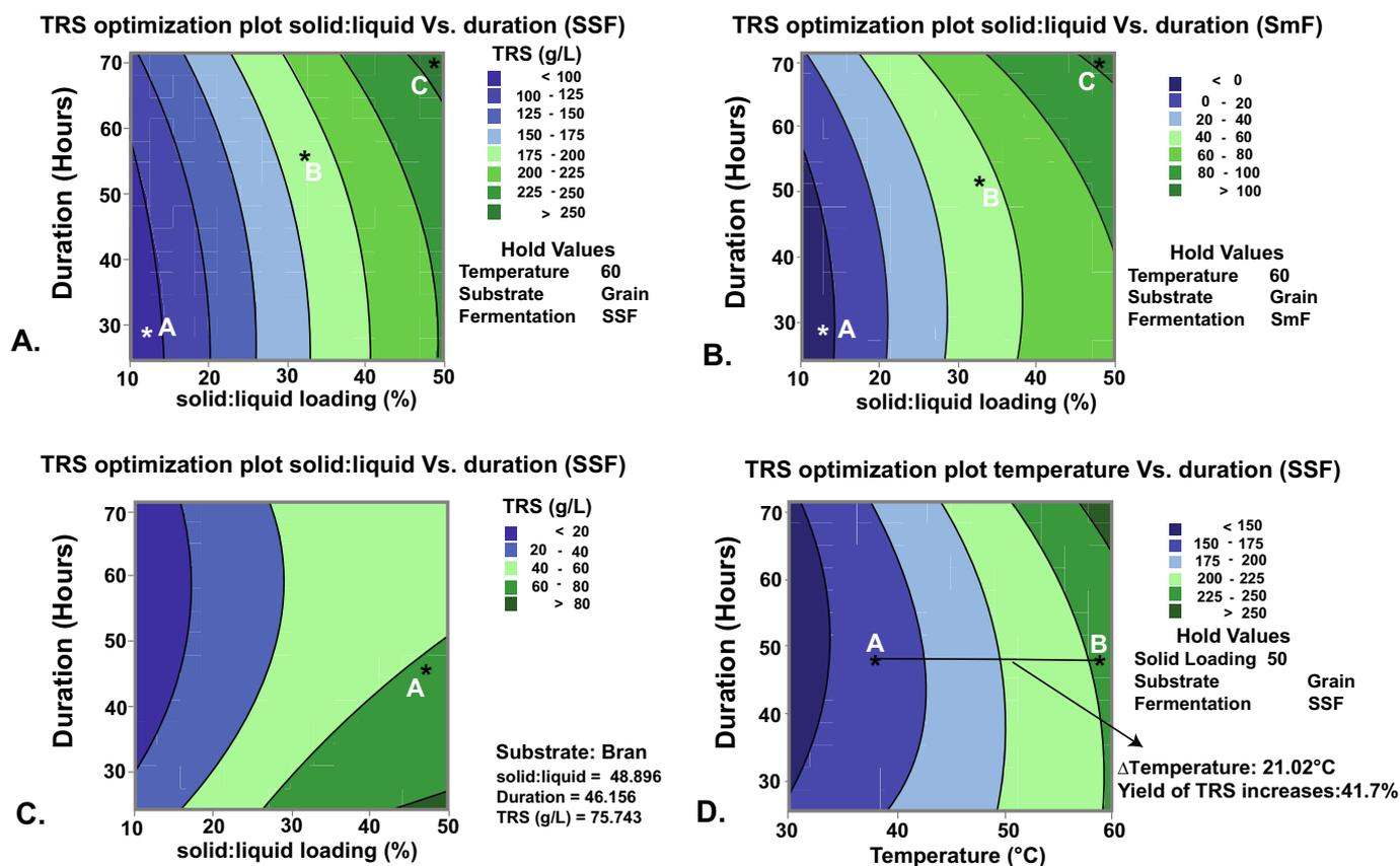
Fig. 10. Contour plots showing the interaction (A). duration vs. solid: liquid using SSF (grain) (B). duration vs. solid: liquid using SmF (grain), (C) duration vs. solid: liquid using SSF (bran), (D). Duration vs. temperature using SSF (grain). [Note: Grain PSD 1.18–0.6 mm and Bran PSD <0.6–0.3 mm were used; solid: liquid (%) was calculated as (w/v) ratio].
