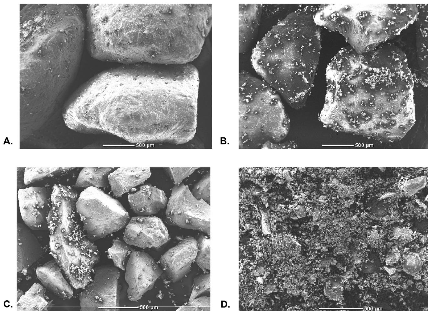
**Fig. 1.** Scanning electron microscopy (SEM) of sorghum grain ( $40\times$  magnification) (A) PSD  $>1.18$  mm (smooth surfaces with high void spaces). (B)  $1.18\text{--}0.6$  mm (fractured surface with attached fine particulate matter). (C)  $<0.6\text{--}0.3$  mm (fractured surface and irregular shapes). (D)  $<0.3$  mm (highly compact with minimal void spaces).
