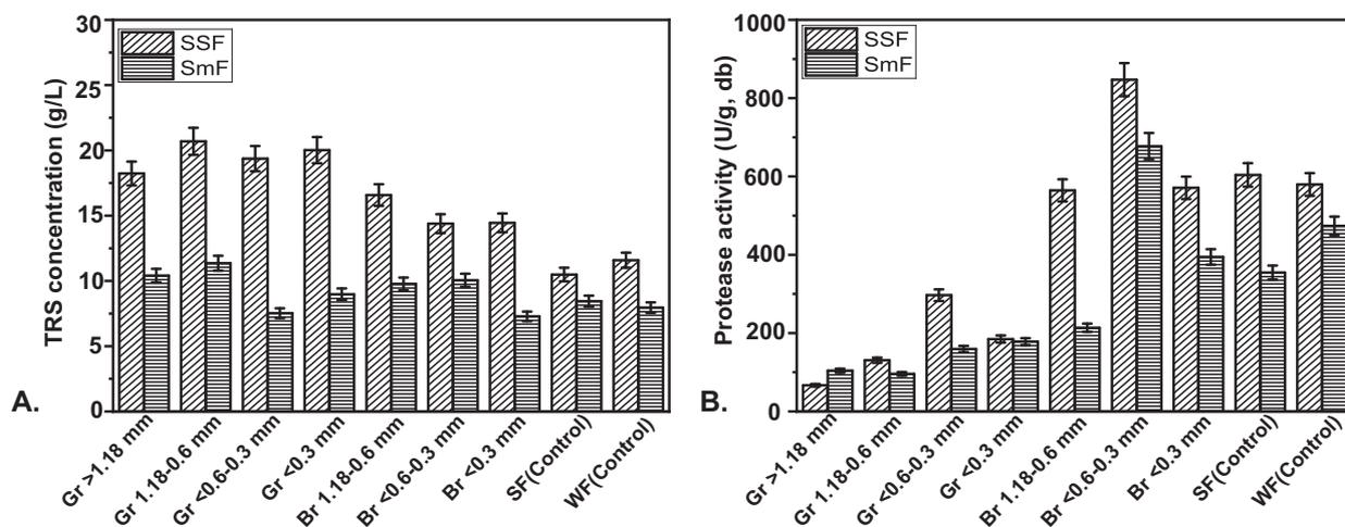
Fig. 6. SSF vs SmF yield analysis using *A. oryzae*: (A) Total reducing sugars (TRS) production, and (B) protease activity. [Note: solid-liquid ratio (SSF): 1:8 (w/v)].
