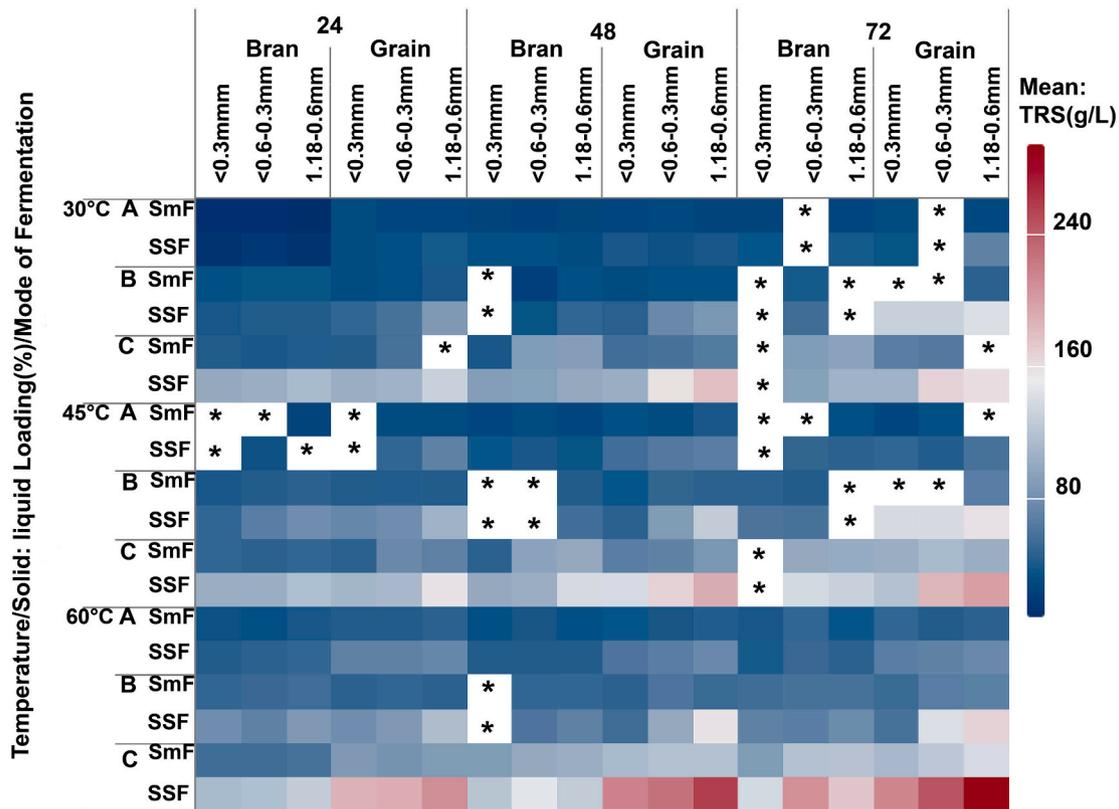
Fig. 12. Heatmap plot for parameter optimization and effects for TRS yield [\*: Data not available; A: 1:10 (w/v); B: 1:4 (w/v); and C: 1:2 (w/v), PSD: particle size distribution].
