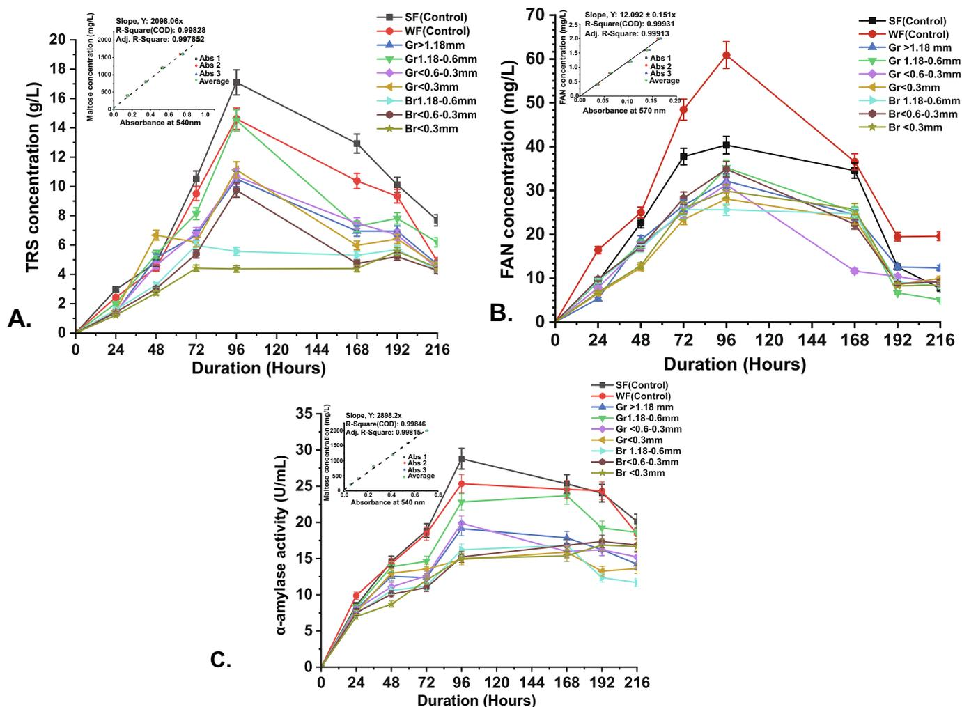
Fig. 4. Trend analysis of *Aspergillus awamori* in solid-state fermentation (SSF) for (A) TRS production, (B) FAN production, and (C)  $\alpha$ -amylase production. [SF: commercial sorghum flour; WF: commercial wheat flour; Gr: grain and Br: bran] [Note: Solid-liquid ratio: 1:20].
