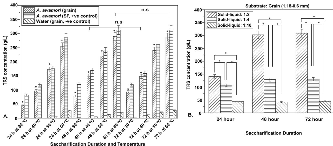
Fig. 9. Optimization of TRS yield using SSF: (A) effect of saccharification duration and temperature [\*: statistically significant, where  $p < 0.001$ ; n.s: not significant; +ve: positive; -ve: negative. Significance testing was performed within the sample group (grain) only]. (B) Effect of solid: liquid loading [\*: statistically significant,  $p < 0.001$ ].
