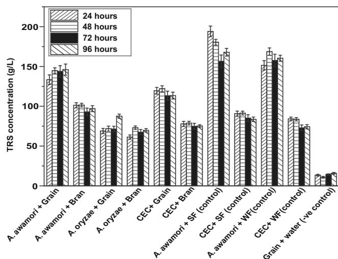
**Fig. 7.** Comparison of saccharification efficiency between in situ produced enzymes and commercial enzyme cocktails based on total reducing sugar (TRS) production at 60 °C. [Note: Grain: PSD 1.18–0.6 mm; Bran: PSD <0.6–0.3 mm; CEC: commercial enzyme cocktail; SF: Commercial sorghum flour used as a positive control; WF: commercial wheat flour used as a positive control, -ve: Negative].
