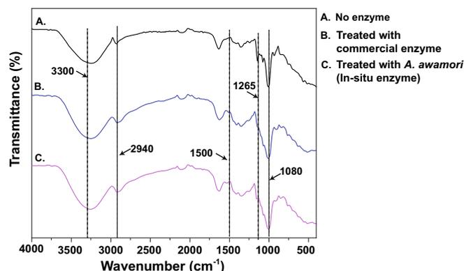
**Fig. 8.** FTIR spectra of sorghum grain [untreated grain (A. black line), grain treated with commercial enzymes (B. blue line), and grain treated with in situ enzyme produced by *Aspergillus awamori* (C. pink line). The x-axis represents wavenumber ( $\text{cm}^{-1}$ ), and the y-axis represents transmittance (%)].
