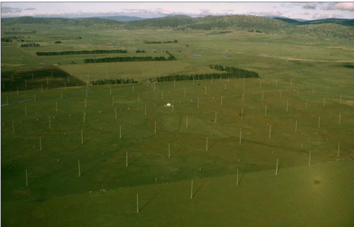
Figure 9: An aerial photograph of most of Reber's Bothwell array taken in 1965, showing the 20.4-m high poles that supported the dipoles, and the small white central receiver hut (courtesy: Estate of Grote Reber).
