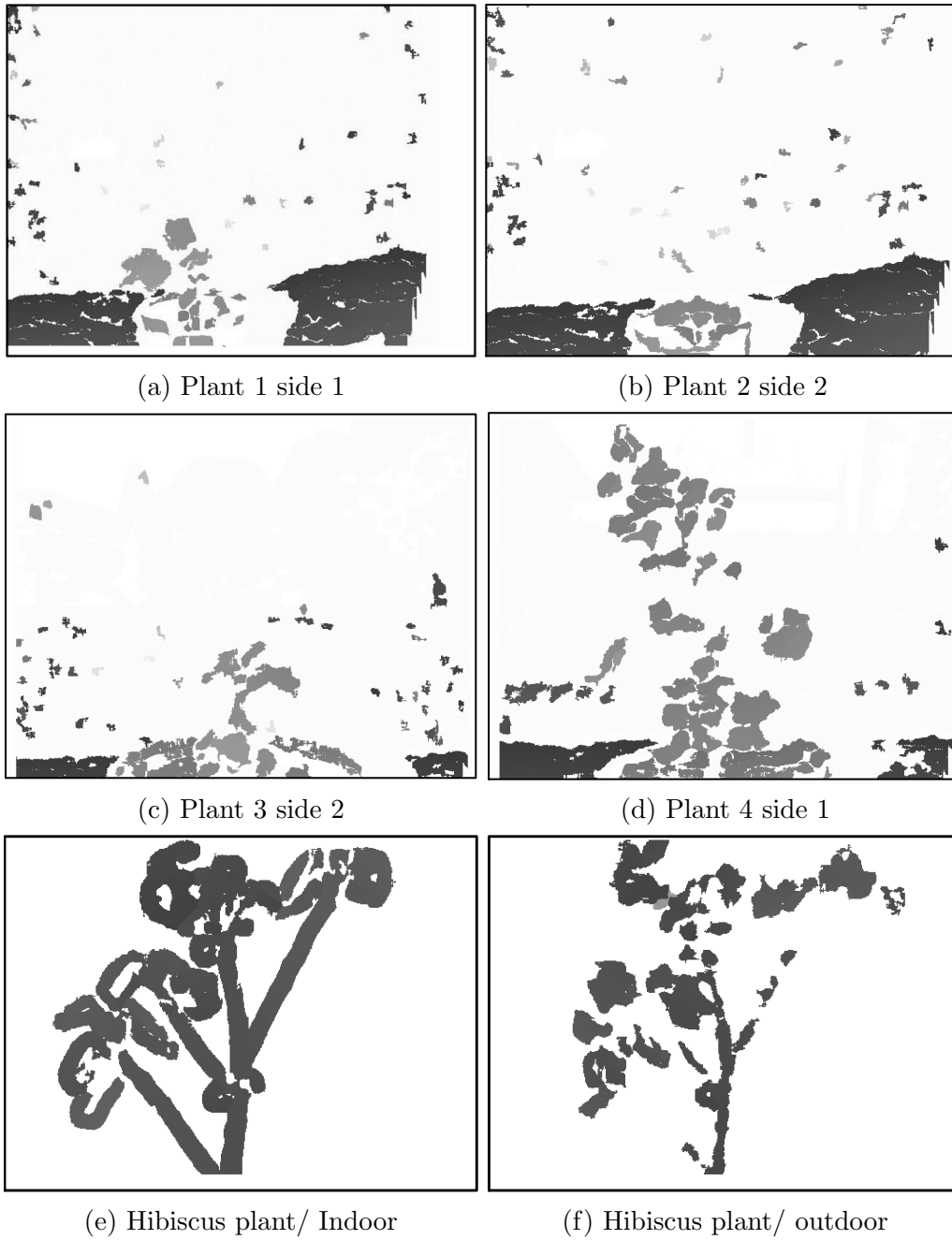
Figure 4.3: Disparity map for the six selected cotton and hibiscus plants. (a), (b), (c) and (d) cotton plants in sunny condition. (e) and (f) Hibiscus plant in indoor and outdoor (sunny) conditions.
