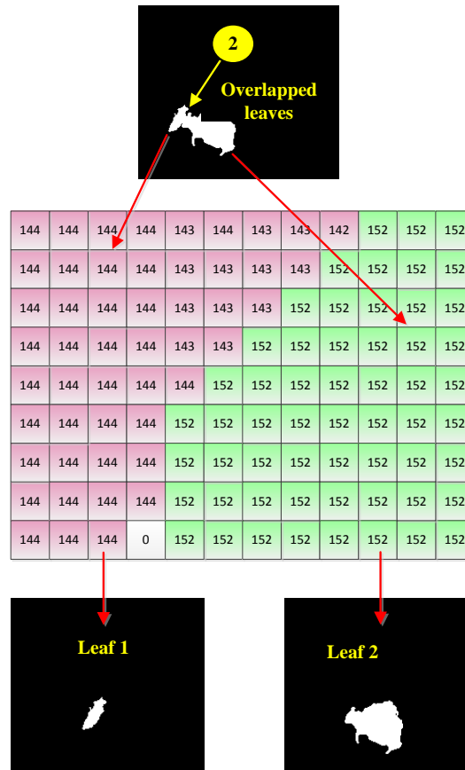
Figure 4.20: Two overlapping leaves (area 2 of Plant 3) and their separation process using GDS technique. The top image shows the overlapping leaves. The disparity map declares the distinct difference between pixels. The lower images present the results after separation.
