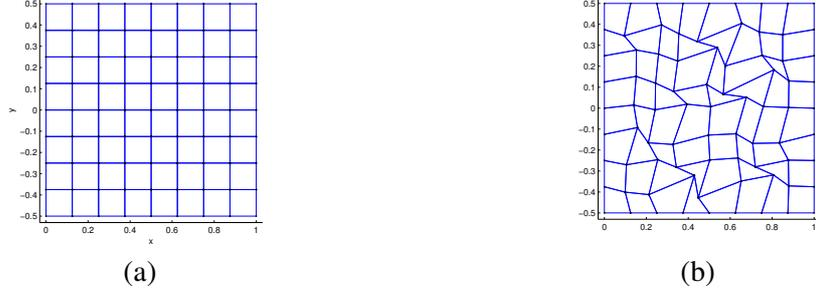
Figure 3. Typical meshes of a piezo-strip: (a) regular elements and (b) irregular elements.
