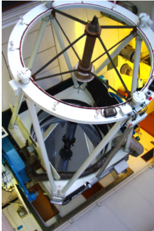
Figure 3.2: 2.3-m telescope with mirror cover open. Echelle spectrograph is located at Nasmyth focal station B on left of photo.
