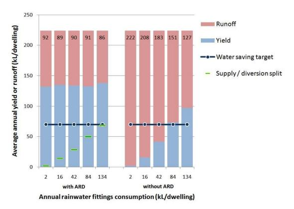
Figure 7 Rainwater harvesting dual performance with and without ARD, for a connected roof area of 150 m<sup>2</sup>, in Caloundra and with performance by consumption scenario
