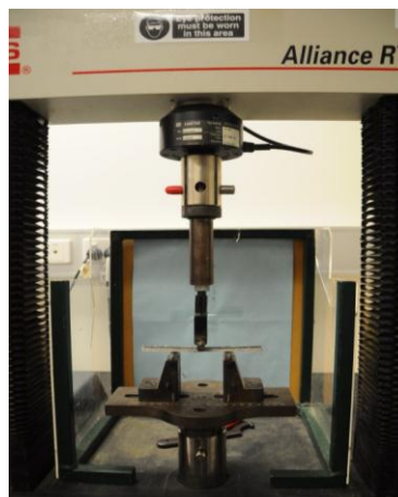
Figure 5.24. MTS Alliance RT/10 machine as used for flexural and ILSS tests.
