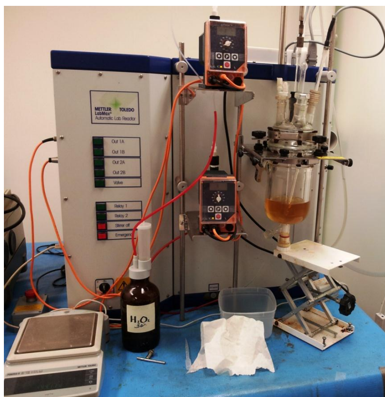
Figure 3.3. Acrylation reaction in a Mettler Toledo LabMax reactor.
