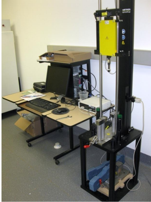
Figure 5.2. Instron Dynatup M14-5162 as used for Charpy impact tests.
