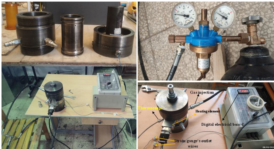
Figure 6 | Pressure cell view during the saturation of the coal sample with CO 2 .
