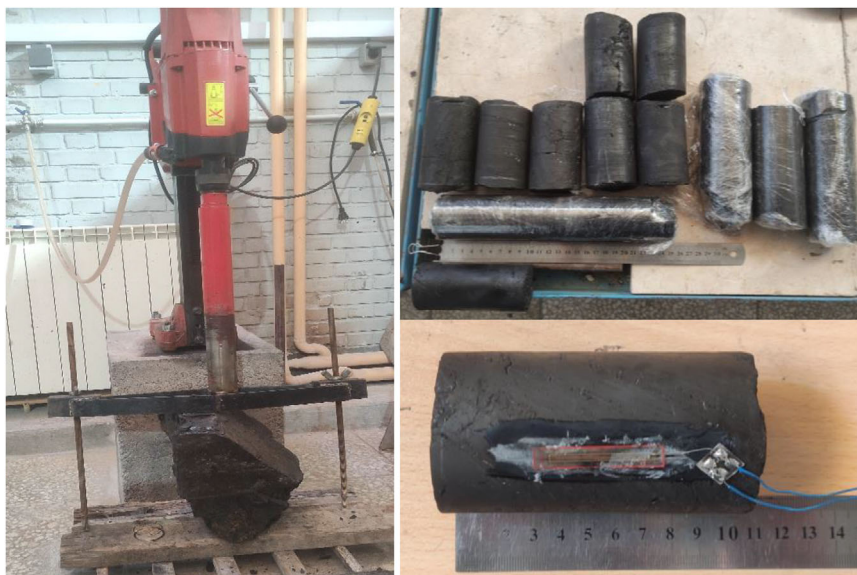
Figure 4 | Preparation stages of coal sample for testing.
