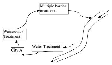
Figure 2: Planned Indirect Potable Reuse
