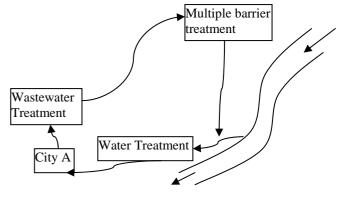
Figure 3: Direct Potable Reuse
