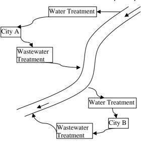
Figure 1: Unplanned Indirect Potable Reuse
