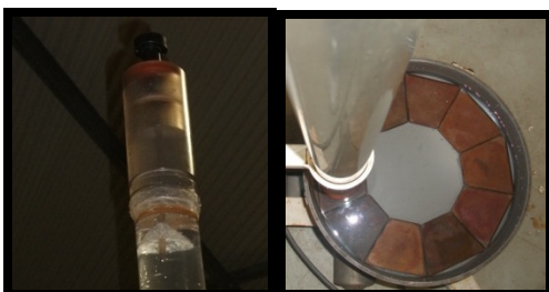
Figure 2: Settling column, Turntable with sampling tray
