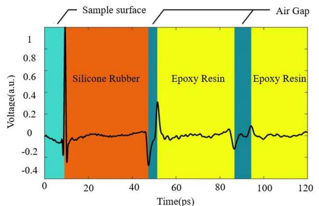
**FIGURE 12** Relationship between the deconvoluted waveform and the defects using THz-TDS [83].
