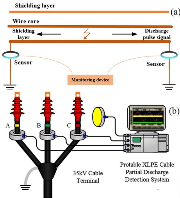
**FIGURE 7** Electromagnetic coupling detection of partial discharge for cable and cable terminals. (a) Schematic diagram and (b) field test diagrammatic sketch.
