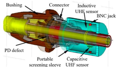
**FIGURE 6** Partial discharge monitoring for high-voltage cable joints based on the ultra-high frequency (UHF) method [31].
