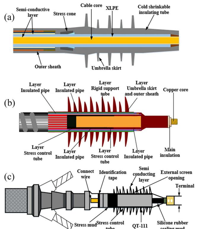
**FIGURE 1** Structure of cable terminal used in (a) distribution power systems, (b) electric multiple units (EMUs), and (c) wind farms.
