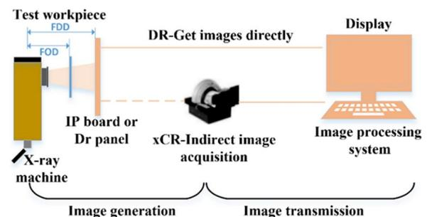
FIGURE 10 X-ray imaging principle.
