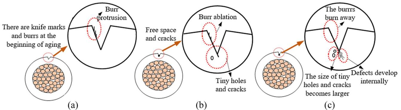
FIGURE 4 Illustrative diagram of knife incision defect. (a) No deterioration stage, (b) intermediate stage of deterioration, and (c) later stage of deterioration [11].
