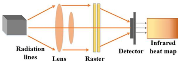
FIGURE 9 Schematic diagram of cable fault using infrared (IR) sensors.
