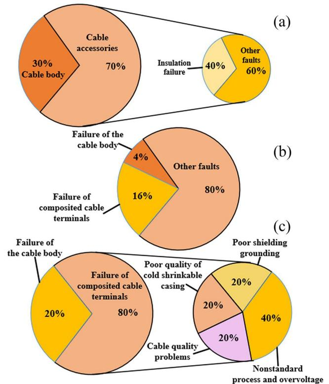
**FIGURE 2** Cable fault statistics for (a) distribution systems (b) electric multiple units (EMUs), and (c) renewable energy farms.
