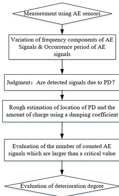
**FIGURE 11** Cable terminal degradation diagnostic procedures using the Acoustic emission (AE) technique [80].
