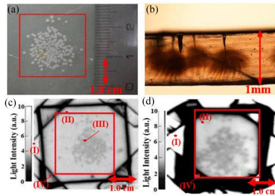
**FIGURE 13** Views of the sample with water trees. (a) A surface view was taken by a digital camera. (b) A cross-sectional view by a polarisation microscope. (c) THz imaging of the sample with water trees. (d) THz imaging results were obtained by scanning the light intensity of reflected THz light pulses over the surface of a polyvinyl chloride sheath [86].
