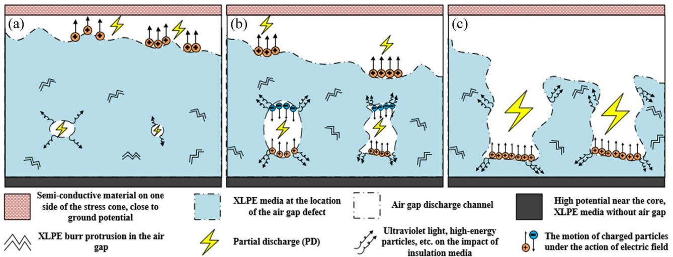
FIGURE 3 Illustrative diagram of discharge development caused by air gap defects: (a) the first stage, (b) the second stage, and (c) the third stage [9].
