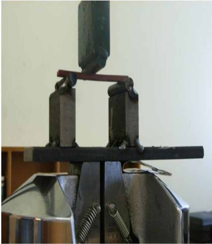
Figure 2: Three-point bending test on flexural specimen
