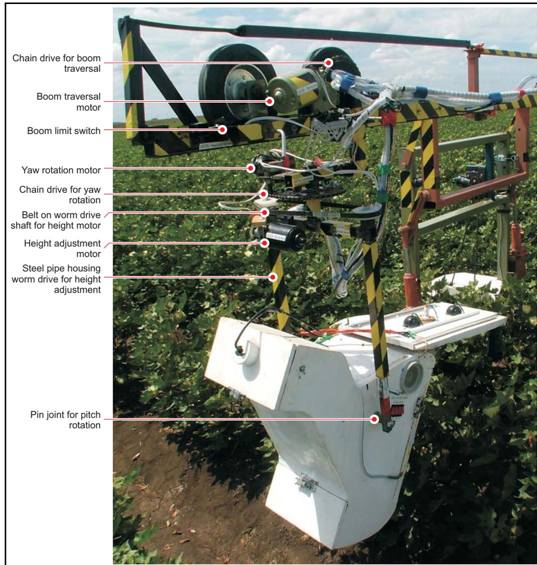
Figure 3.16: Mechanical joints for camera enclosure's automatic conveyance. A mechanical drawing of the drive system is included in Appendix B.
