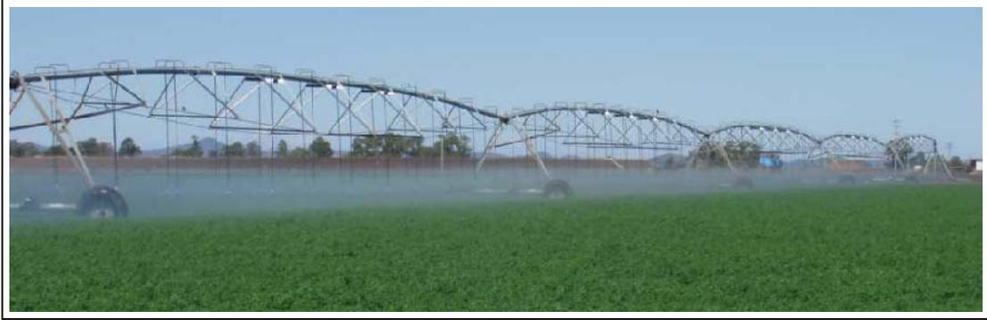
Figure 1.1: Five spans of a large mobile irrigation machine (LMIM) (here, a centre pivot).
