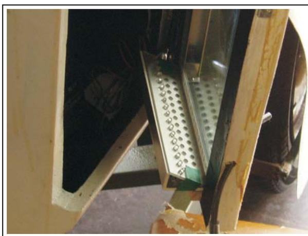
Figure 3.7: One row of LEDs installed in the hinged front window of Mark 4.
