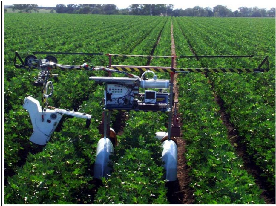
Figure 3.15: Automatic conveyance of camera enclosure in a cotton crop.
