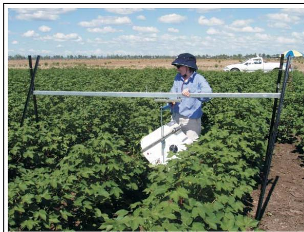
Figure 3.14: Manually moved camera enclosure in a cotton crop.
