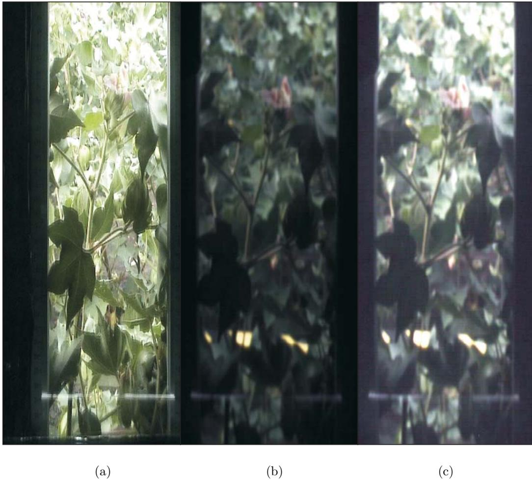
Figure 6.7: Images captured simultaneously of a single plant from Data Set 5, showing effect of a narrow depth of field: (a) image captured from Sony DV camcorder (CCD image sensor), with infinite depth of field; (b) image captured from Prosilica firewire camera (CMOS image sensor), with lensing for a narrow depth of field; and (c) contrast enhanced version of image (b).
