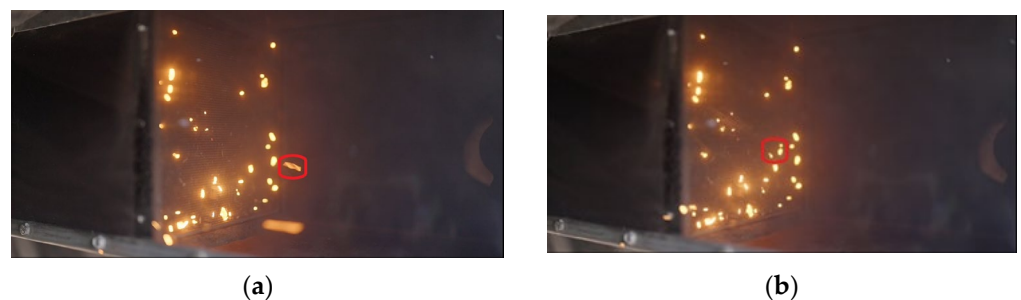
Figure 10. shows splitting mechanism, (a) approaching firebrands, (b) firebrands split into three smaller glowing firebrands at approaching side of the screen (Stainless Steel Wire and Mesh Pty Ltd. [17]).
