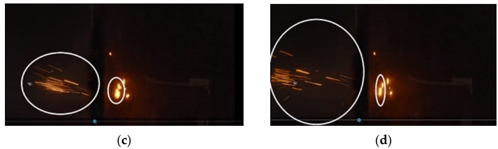
Figure 11. Shattering process, (a) two approaching firebrands, (b) two firebrands hit the mesh and producing tiny secondary firebrands, (c) generated tiny secondary firebrands, and (d) movement of tiny secondary firebrands and the change of the sizes of the two original firebrands (Stainless Steel Wire and Mesh Pty Ltd. [17]).
