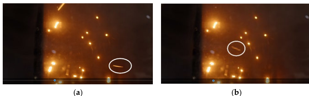
Figure 8. A firebrand passes through the mesh without any contact, (a) approaching firebrand, (b) firebrands after passing the mesh (Stainless Steel Wire and Mesh Pty Ltd. [17]).
