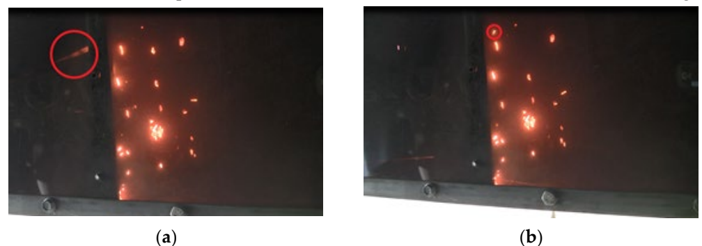
Figure 16. Deceivingly large firebrands at the exit side of the mesh taken by a camera with a speed of 250 frames per second (a) a firebrand with an apparent cross-section greater than the opening of the mesh at the exit of the mesh, and (b) the previous frame shows the of the actual needle shape of the firebrand in a). (Stainless Steel Wire and Mesh Pty Ltd. [17]).
