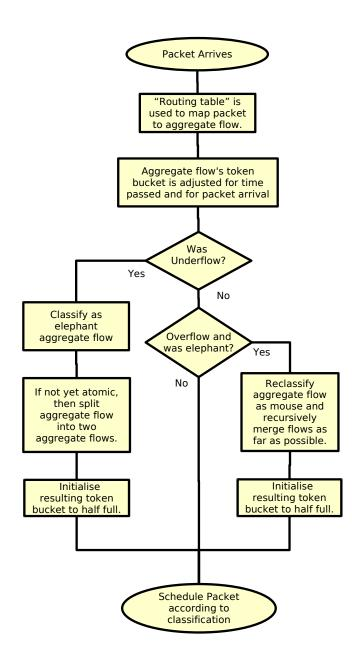
Fig. 1. The per-packet algorithm
