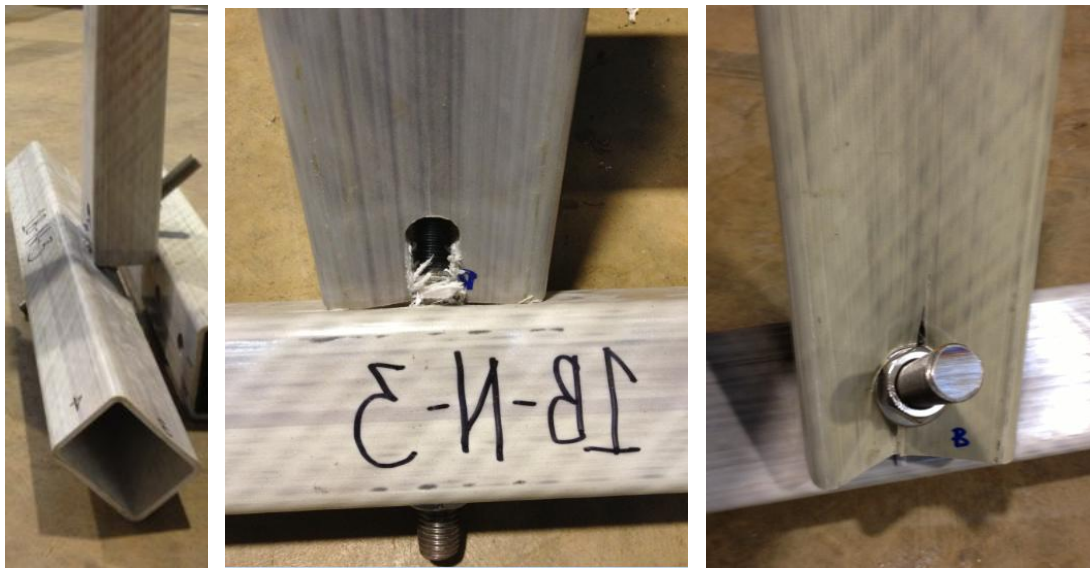
Figure 5. Failure modes of 1B specimens
