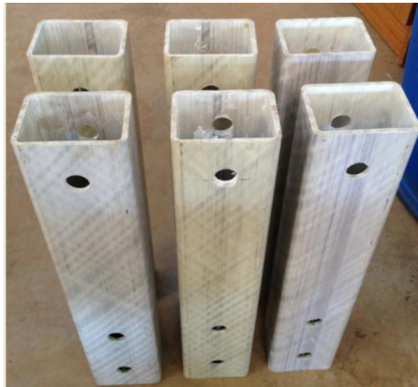
Figure 1. Disassembled specimens of pultruded GFRP closed profile.
