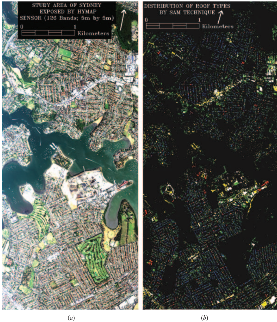
Figure 4. (a) HyMap image (RGB 2,17,47) over study area of Concord Bay, Sydney. (b) Classified (SAM) HyMap image. Colours indicate roof types as follows: blue = terracotta; red = concrete; white and yellow = metal; green = slate.
