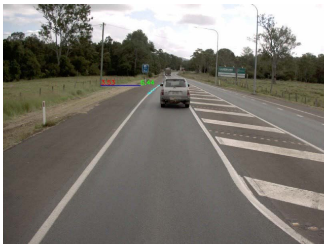
FIGURE 7. In this figure, the distance calculated by the proposed method is shown in green, and the distance from the lane-line method is shown in red.
