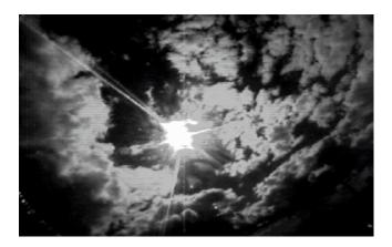
**Figure 3** CCD image taken by the SCSC on the  $20^{th}$  October 1997 at 2:38 PM. This cloud configuration produced the greatest enhancement of 30 %. This case had a SZA of 38.7 °, a CAFOV of 96.3 %, and an ozone level of 330 DU.
