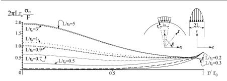
Fig. 5 The variation of tensile stress throughout a disc subjected to the loading defined by (2), when  $\nu = 0.25$  and  $2\alpha = 10^{\circ}$
