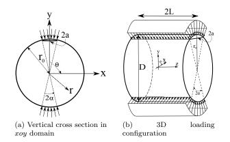
Fig. 1 Cross sections of a standard Brazilian disc subjected to diametrically opposite radial loads
