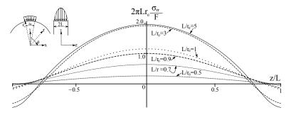
Fig. 4 The variation of radial stress at the centre  $(\sigma_{rr, r=0, \theta=\pi/2})$  of a solid disc subjected to parabolic loading along its thickness defined by Eq. (2), when  $\nu = 0.25$  and  $2\alpha = 10^{\circ}$
