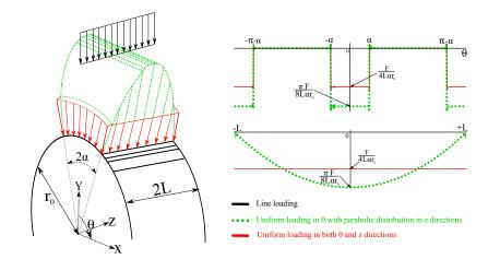
Fig. 2 The loading types comparatively considered
