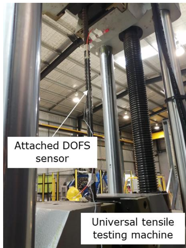
Figure 5.25: Experimental setup of rebar testing
