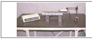
Figure 5 The layout for the 'Surface Roughness' experiment and the workpiece used in the testing.
