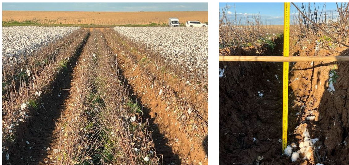
Fig. 1 Large rutting caused by a cotton picker while harvesting on soft soil in 2024 near Griffith (New South Wales, Australia). The cotton picker was fitted with dual tires (520/85R42-R1, average wheel load: 5.43 Mg, inflation pressure: 2.5 bar) on the front axle and single tires (520/85R34-R1, average wheel load: 8.25 Mg, inflation pressure:
