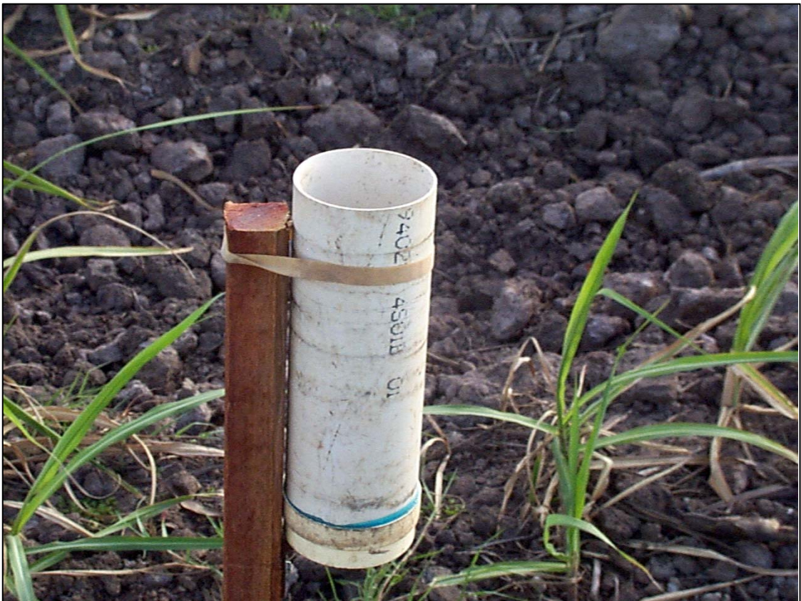
Figure 4-1 Catch can - 90 mm PVC pipe with glued end caps
