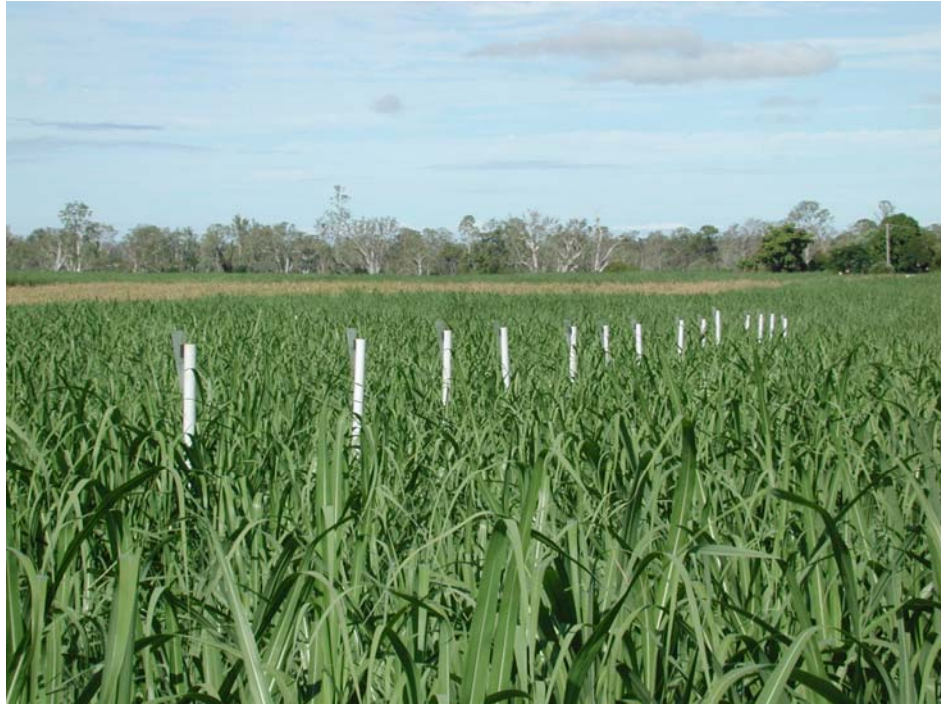
Figure 6-1 Catch cans arranged in standing leg test
