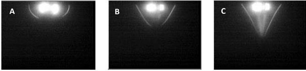
**Figure 2.3:** Formation of the Taylor cone. A) Voltage starting, B) Voltage increasing, C) Equilibrium between surface tension resulted in electrostatic force (Zufan, 2005).
