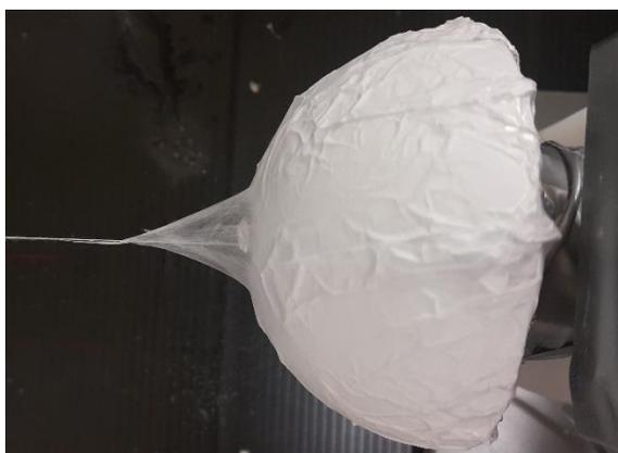
**Figure 4.2:** Triangular spinning of electrospun nanofiber.
