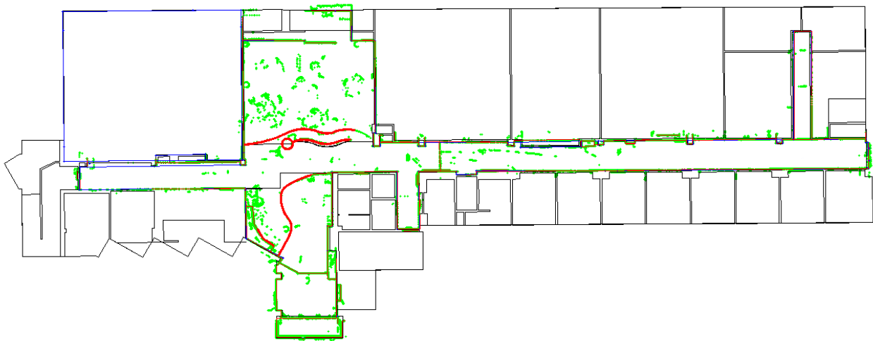
Figure 8: The three data sets overlapping. Black represents the original drawings, blue was captured by the survey, green is the raw point cloud and red is the extract plans from the point cloud.
