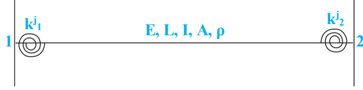
Figure 1. Modeling semi-rigidly connected frame element with rotational springs
