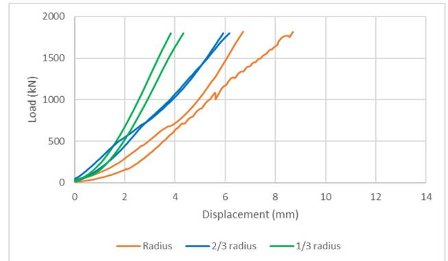
Figure 7. Load deformation curves for cementitious grout
