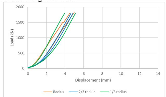
Figure 8. Load deformation curves for crane rail
