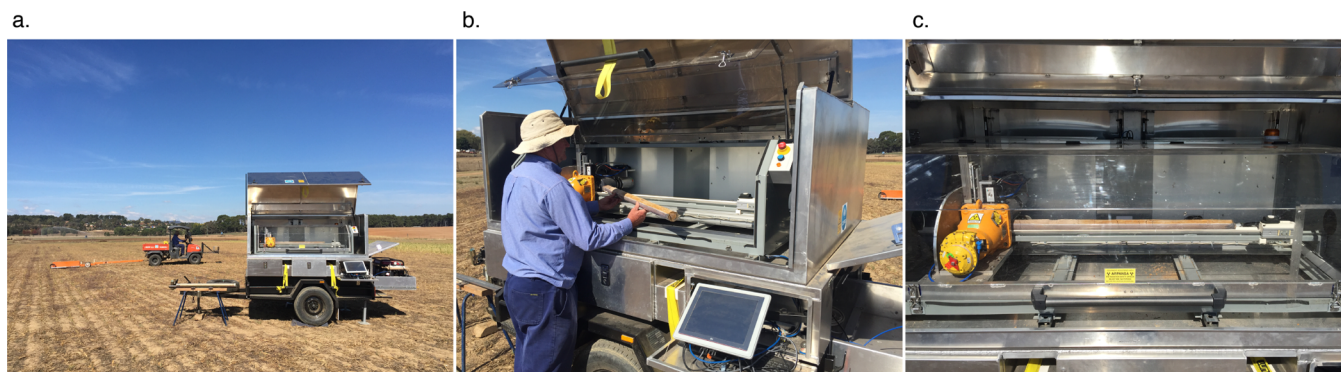
Figure 3. SCANS field-deployable core sensing system (CSS): (a) the SCANS sensing systems at a field site, (b) an operator loading a soil core on the CSS, and (c) the core sensing system.
