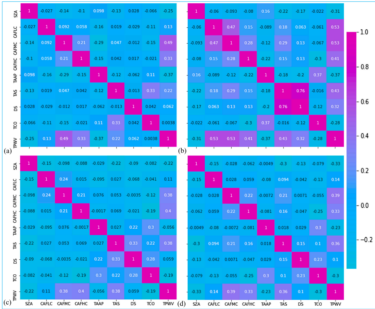
Fig. 4. Second phase of feature selection using a color-coded heat map highlighting a visual overview of low, average and high correlation (r) of the predictor inputs considered for (a) Darwin, (b) Alice Springs, (c) Townsville and (d) Emerald; where any two variables having high r (preferably r > 0.8 or r < -0.8 for this study) are regarded redundant and one of them is eliminated from the design phase of the hybrid explainable EJH-X-DNN model.
