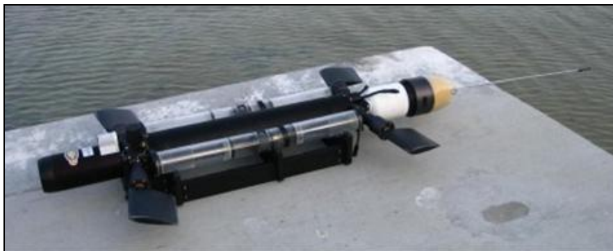
Fig. 7. iRobot™ 'Transphibian' foil-actuated swimming robot (from www.irobot.com )
