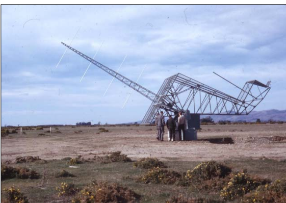
Figure 8: The tracking antenna used for solar noise monitoring (courtesy: University of Canterbury).
