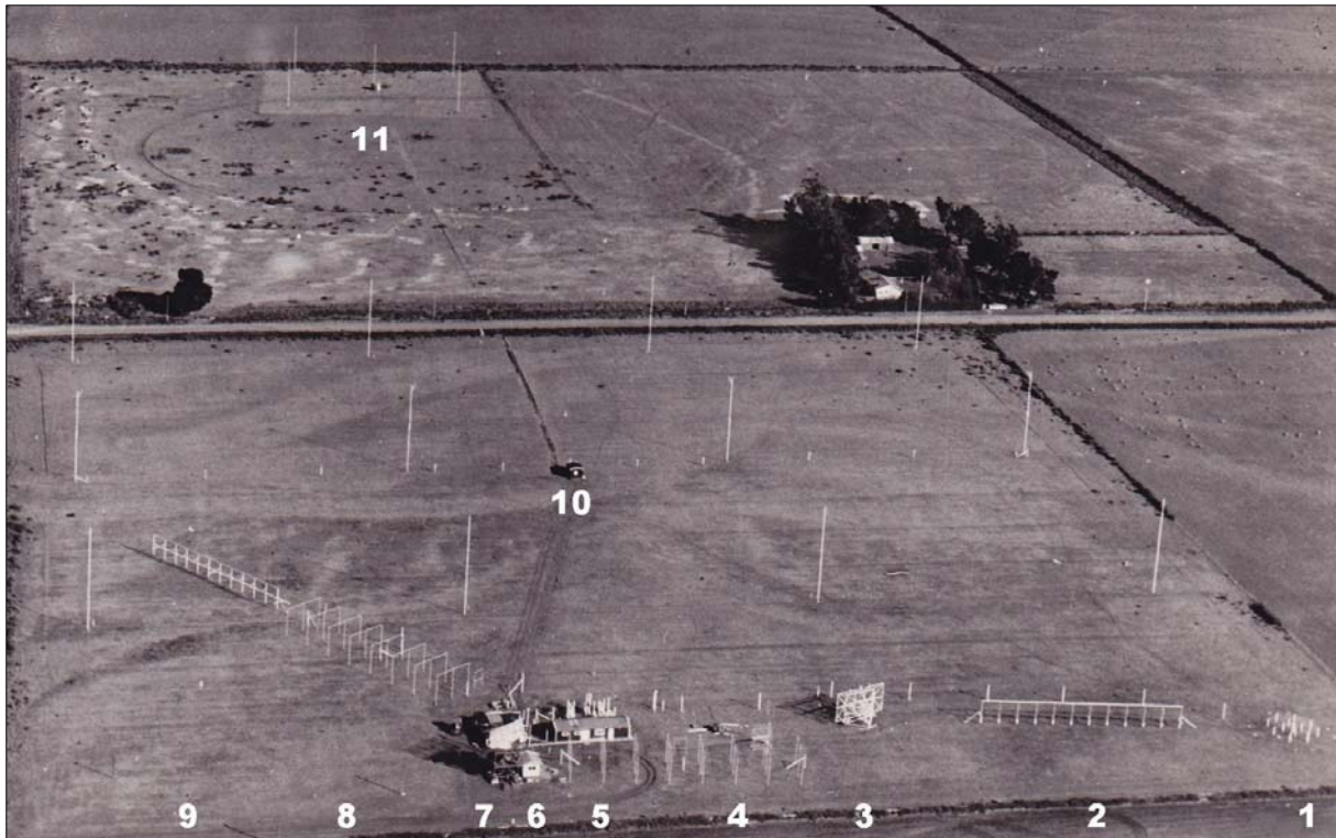
Figure 7: Rolleston research station aerial view ~1960. Features are as indicated: 1. Crossed dipoles for all-sky meteor surveys; 2. Array for radiant determination; 3. Broadside rotating (360°) array (the first array on the site); 4. Broadside array of eight Yagis each of 7 elements for radiant determination; 5. Receiver and recording hut (black walls); 6. Hut with 200 MHz radar and behind is the CHL rotating antenna; 7. The hut, behind the 200 MHz radar, housing the 69 MHz GL2 transmitter; 8. More Yagis for radiant determination; 9. Additional broadside array for radiants. 10. Broadside transmitting array for the partial reflection atmospheric radar operating on 1.75 MHz. 11. 1.75 MHz circular polarisation receiving array (courtesy: University of Canterbury).
